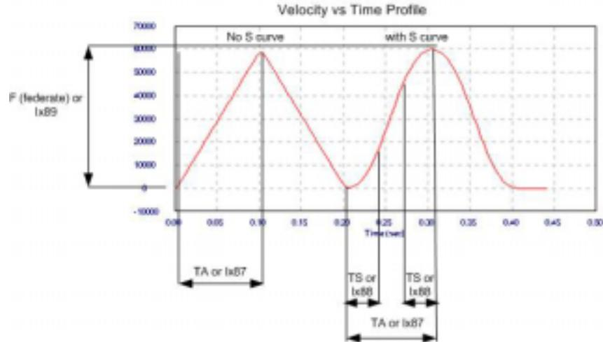
In all cases, if two times the S-curve acceleration parameter is greater than the linear acceleration parameter, then the overall acceleration time will be two times the S-curve acceleration time:
