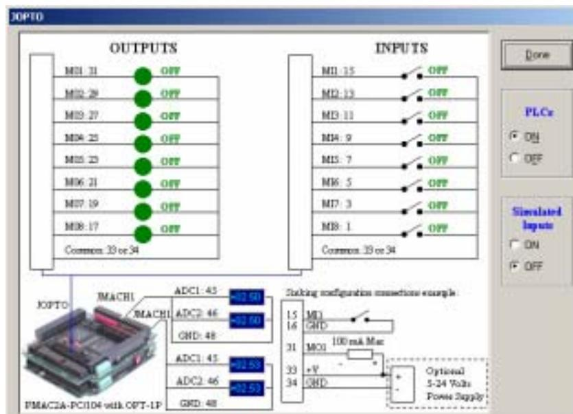
Clicking on the **I/O Port** button on the PLC Programs page will show PMAC's general-purpose digital I/O connector page. This page checks the PLC program example written above.
