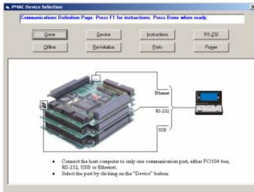
Once PMAC is properly powered and the communications cable has been connected between the host computer and the PMAC, communications can be established. The communications setup screen appears when the program is run for the first time or when the PMAC cannot be found in the previously defined channel of communications. Press the F1 function key for instructions.
