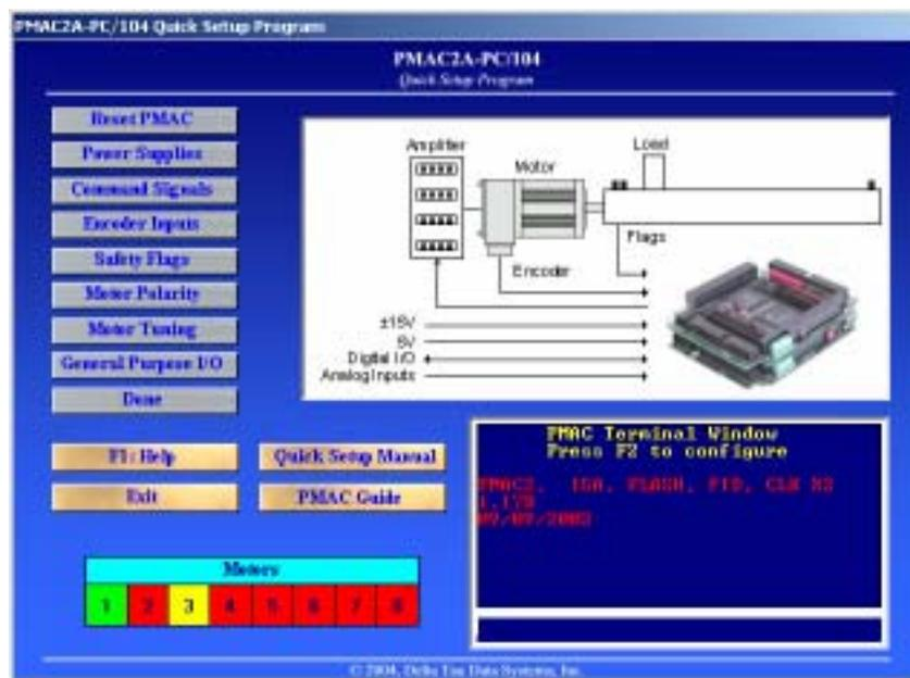
Once communications has been established, the main Setup screen displays. At any time during the execution of this program, press the F1 function key to get instructions for each particular page.
