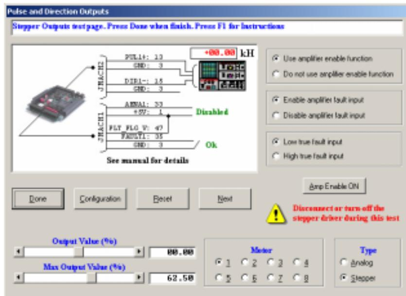
On this page, select the output type for a particular motor to be either analog  $\pm 10V$  or pulse-and-direction stepper outputs. The following is the description for the pulse and direction outputs test.
