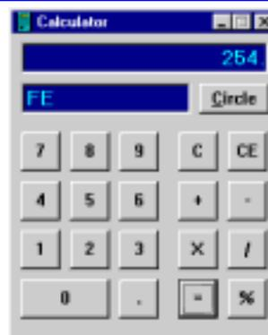
This simple calculator has common arithmetic functions and an automatic decimal to hexadecimal conversion for every number entered. The hexadecimal field can be edited to obtain hexadecimal to decimal conversions as well.
