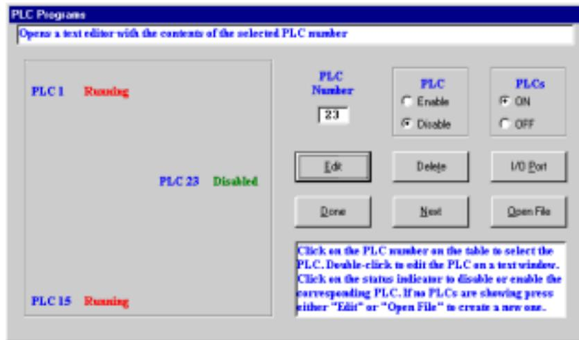
PMAC is not only an excellent motion controller, but it can perform PLC operations. The 32 different PLC programs are similar to motion programs, but they run independently of motion programs and of other PLCs.
