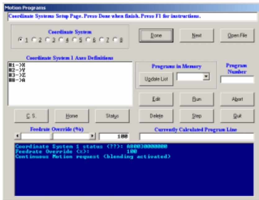
From this centralized screen, a motion program can be written, edited, run and debugged. The coordinate system definitions and the status portion of the screen are used for indication and diagnostics only.
