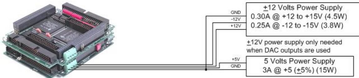
PMAC2A-PC/104 stack with ACC-1P Axes Expansion Board
