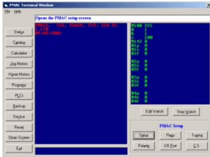
After PMAC has been configured properly, this terminal screen becomes the main operating screen from which every previously described function can be accessed easily.
