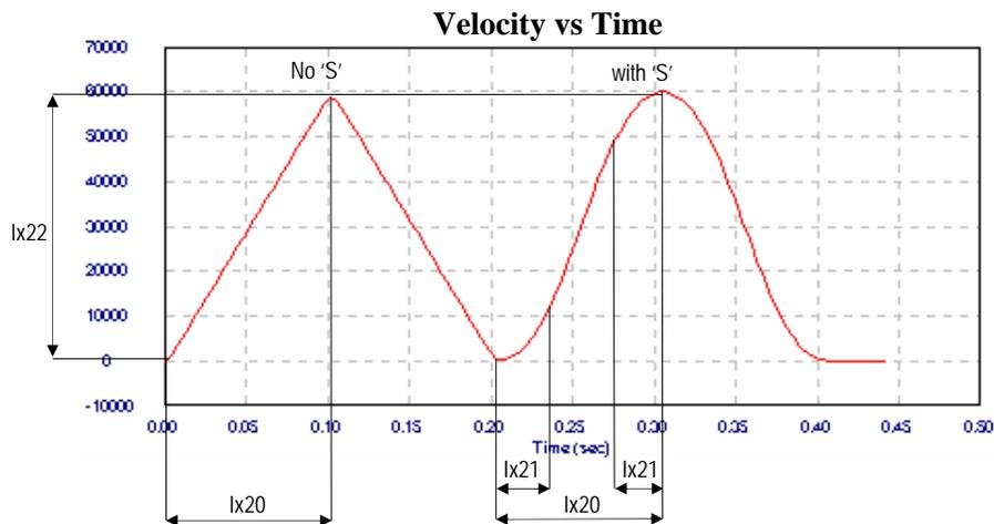
The acceleration portion of a jog-programmed move is controlled by two time parameters in units of milliseconds. In the case of jog or homing commands, these two parameters are I-Variables Ix20 and Ix21. Ix20 determines the overall acceleration time which is the total time required for any change in velocity. Ix21 determines the portion of the overall acceleration ramp that is performed in S-curve mode.
