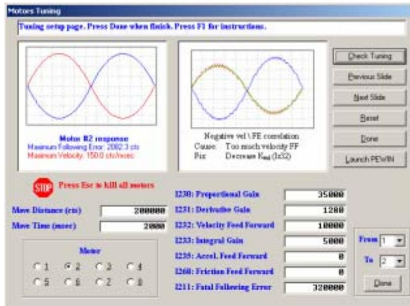
The tuning process is the definition of the PID loop parameters and the confirmation that PMAC can move the motors in closed loop with limited following error. The basic tuning procedure provided by the PMAC Quick Setup program might be limited in some cases to achieve an optimum tuning performance, but would allow, nevertheless, moving the motors in closed loop. For a more accurate tuning procedure, use a more sophisticated program like PEWIN or P2SETUP, both provided separately.
