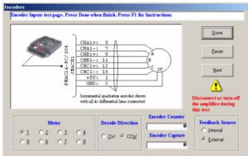
For a proper motion control process, PMAC needs to know motor position at all times. The encoder feedback provides this information. The encoder used for a typical application has the following characteristics:
