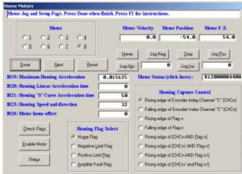
Home commands allow establishing a physical point of reference for all programmed moves. If no home procedure is performed for a particular motor, the zero physical point of reference of that motor will be located at the point where it is found on power-up or reset.
