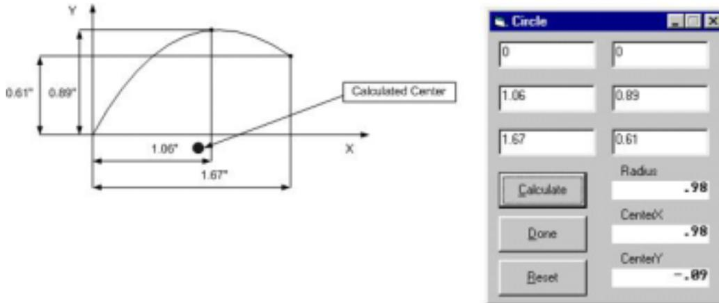
This function calculates the center and radius of any circular path, given the coordinates of three non-aligned points that belong to it. This is useful when programming PMAC in circular interpolation mode.
