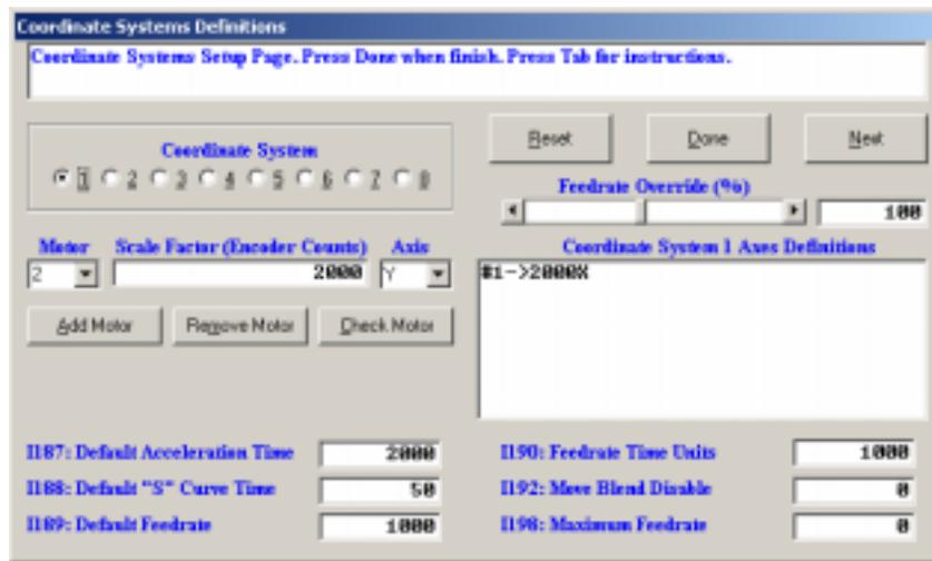
Before running a motion program, a coordinate system must be defined. A coordinate system consists of one or several motors that will be controlled in a coordinate fashion from a motion program.
