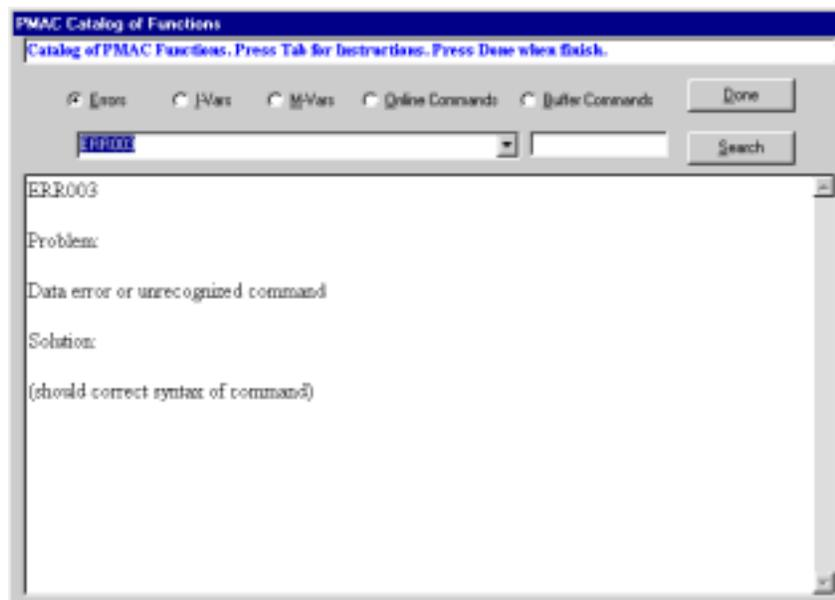
This function, accessible from the **F1 Help** command, allows searching for the description of any PMAC setup variable or command. The **Search** button will list all the entries based on a particular entered search key. This window can be kept open at all times for easy reference to each command in every part of the setup process.
