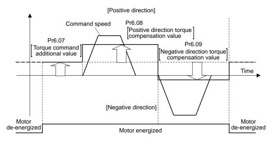
The friction torque compensation will be added in response to the entered positional command direction as shown below.
