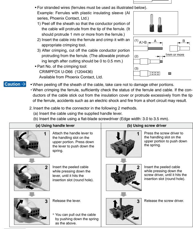
Take off the connector from the Servo Driver before making connection.Insert only one cable into each one of cable insertion slot.
