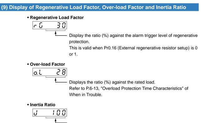
Displays the inertia ratio (%) .
