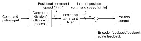
\*4 Command positional deviation is the deviation with respect to the command pulse input and the encoder positional deviation/ full-closed positional deviation is the deviation at the input section of the positional control, as described in the figure below.
