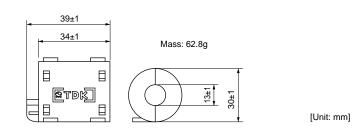
**Remarks** is Fix the signal line noise filter in place to eliminate excessive stress to the cables.
