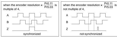
• In case of the 5-wire, 20-bit incremental encoder, the signal sequence might not follow the above fig. until the first Z-phase is fed out. When you use the pulse output as the control signal, rotate the motor one revolution or more to make sure that the Z-phase is fed out at least once before using.
