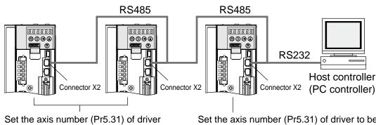
Set the axis number (Pr5.31) of driver to be connected through RS485 to a value in the range 1 to 31. Set the axis number (Pr5.31) of driver to be connected to the host through RS232 to 0.
