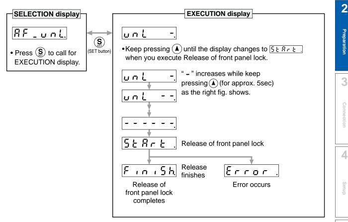
• After release of front panel lock finishes, return to SELECTION display, referring to structure of each mode (P.2-54).
