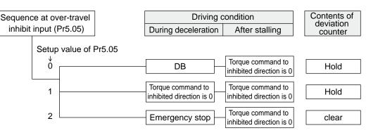
Torque limit value during deceleration will be that of Pr5.11 (Setup of torque at emergency stop) when the setup value is 2.
