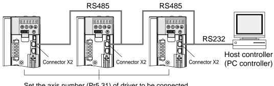
Set the axis number (Pr5.31) of driver to be connected through RS485 to a value in the range 1 to 31.
