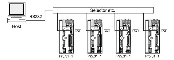
• Set up the module ID of MINAS-A5 to RSW of the front panel. In the above case, you can set any value of 0 to 127. You can set the same module ID as long as the host has no difficulty in control.
