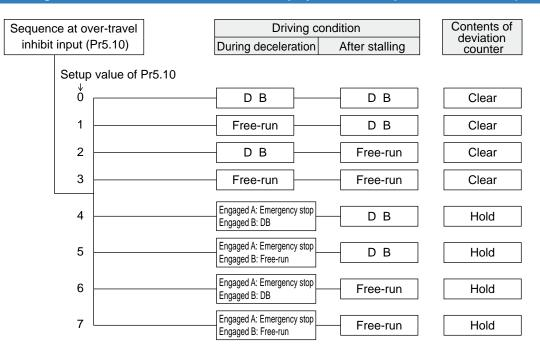
When setup value is within the range 4 and 7, the protection function that supports immediate stop acts according to operation A and the function that does not support acts according to operation B.
