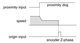
Proximity dog off....Decelerates at an entry of the proximity input, and stops at an entry of the first origin input (Z-phase) after the input is tuned off
