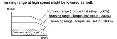
• When you lower the torque limit setup (P0.13 and 5.22),
