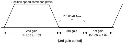
Position loop gain =  $Pr1.00 \times Pr6.06/100$ Speed proportional gain =  $Pr1.01 \times Pr6.06/100$ Time constant of velocity integration, speed detection filter and torque filter directly use the
