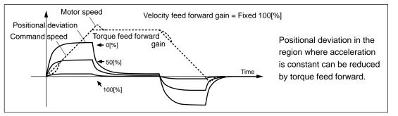
Zero positional deviation is impossible in actual situation because of disturbance torque. As with the velocity feed forward, large torque feed forward filter time constant decreases the operating noise but increases positional deviation at acceleration change point.
