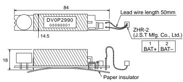
**Caution** This battery is categorized as hazardous substance, and you may be required to present an application of hazardous substance when you transport by air (both passenger and cargo airlines).
