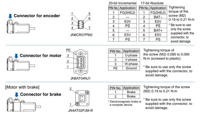
• When the motors of <MSME (1.0 kW to 5.0 kW), MDME, MGME, MHME> are used, they are connected as shown below.
