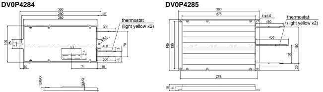
**Remarks** Thermal fuse is installed for safety. Compose the circuit so that the power will be turned off when the thermostat is activated. The thermal fuse may blow due to heat dissipating condition, working temperature, supply voltage or load fluctuation.
