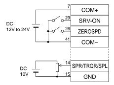
Run with ZEROSPD switch close, and Stop with open
