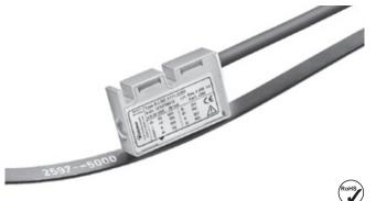
The non-contact incremental magnetic linear measurement system LI20 / B1 - made up of the sensor head LI20 and of the magnetic band B1 - reaches a resolution up to 10 µm with a maximum distance of 1 mm between the sensor and the band.
