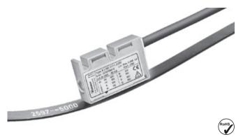
The non-contact incremental magnetic linear measurement system LI50 / B2 - made up of the sensor head LI50 and of the magnetic band B2 - reaches a resolution up to 5 µm with a maximum distance of 2 mm between the sensor and the band.
