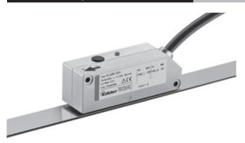
The non-contact absolute magnetic linear measurement system LA50 / BA5 - made up of the sensor head LA50 and of the magnetic band BA5 - reaches a resolution up to 10  $\mu m$  with a maximum distance of 1.5 mm between the sensor and the band.
