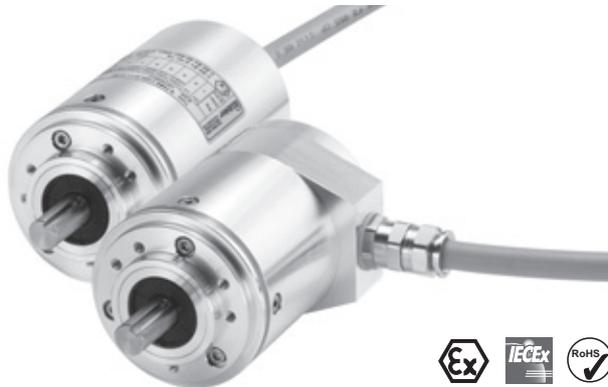
The Sendix 7068 absolute multiturn encoders offer Ex protection in a compact 70 mm seawater resistant housing, with a Profibus interface and optical sensor technology.
