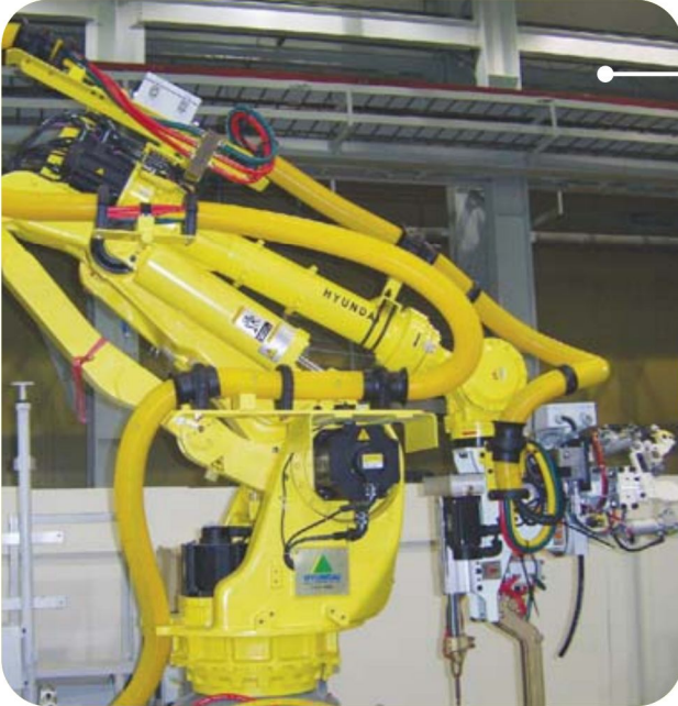
Robo-Kit is designed to prevent the disconnection of cables and minimize interference during operation. 케이블의 단선을 방지하고 간섭을 최소화 시킨 ROBO-KIT
