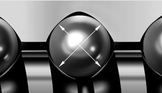
(Contact between ball and Circular-arc Groove)
