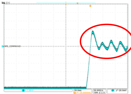
Output offset : 1000 rpm Output scale : 100rpm/V
