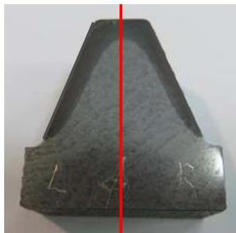
Qualified induction hardening and bad teeth grinding
