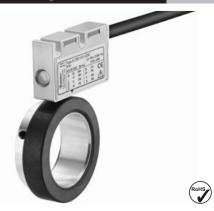
Thanks to its installation depth of only 16 mm, the bearingless magnetic rotary encoder RLI50, comprising a magnetic ring and sensor head, is ideally suited for plants and machinery where space is very tight. The non-contact measuring principle allows for error-free use even under harsh environmental conditions, as well as ensuring a long service life. In contrast to our measuring system RLI20, a single zero pulse is also implemented here.
