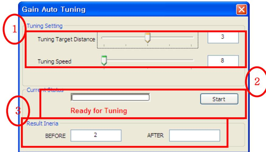
Figure 54- Gain Auto Tuning operation screen
