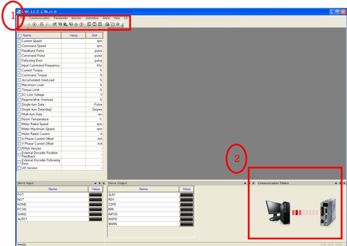
Figure 21 - Communication connection
