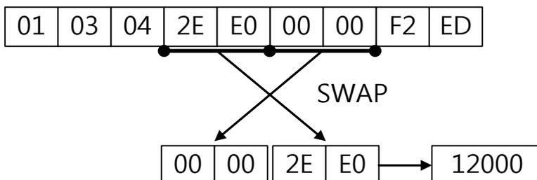
Be cautious with parsing for a 2 byte register since 1 byte for each of the upper and lower parts is swapped. For example, '2E E0 00 00' is swapped and converted into a decimal number, 12000.
