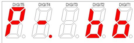
Three digits from Digit 3~1 of the 7-Segment represent the drive status as described below if no servo alarm occurs. In the event of a servo warning occurrence, the warning status display takes precedence over other status.
