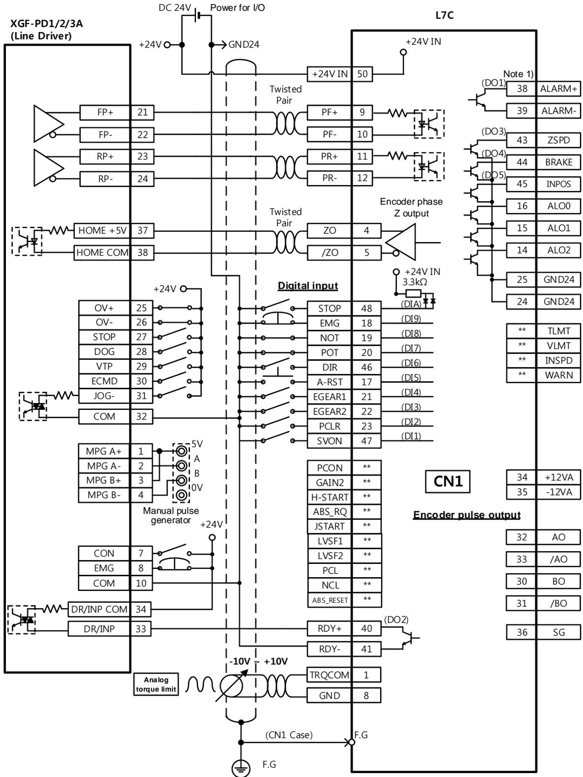
※ This is an example of a wiring diagram for a single shaft. For wiring with 2 or 3 shafts, refer to the pin arrangement for the positioning module.
