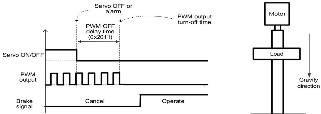
(2) If PWM output is turned off before the brake signal output
