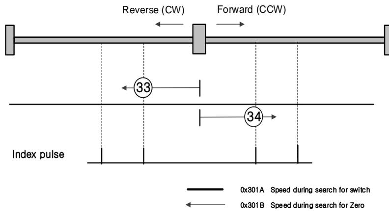
The initial driving direction is reverse (CW) for method 33 and forward (CCW) for method 34. The drive detects the index pulse at the zero search speed.
