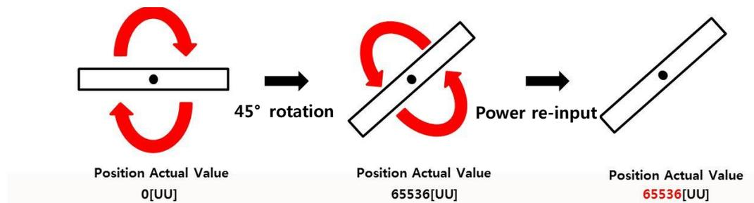
When you set the value to 2, power re-supply resets the multiturn value to 0[revolution] but brings the encoder's singleturn value for the current position and displays it.
