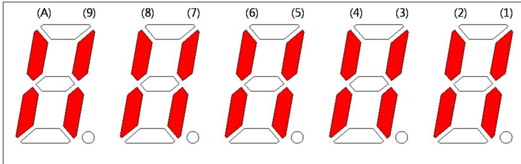
If an LED that corresponds to a contact is turned on/off, it indicates the ON/OFF state of the contact.
