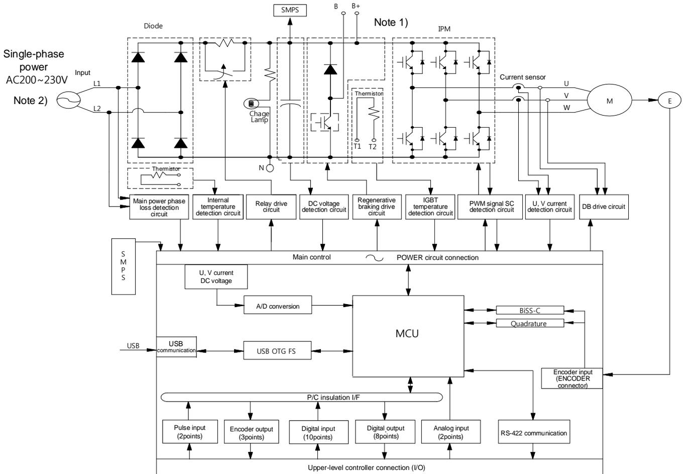
**Note1)** Since there is no internal regenerative resistance, make sure to connect regenerative resistances to B+ and B pins.
