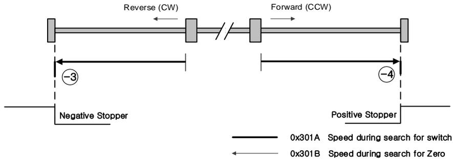
Homing methods -3 and -4 perform homing only by using the stopper. The velocity profile according to sequence is as follows. For more information, see the details below.
