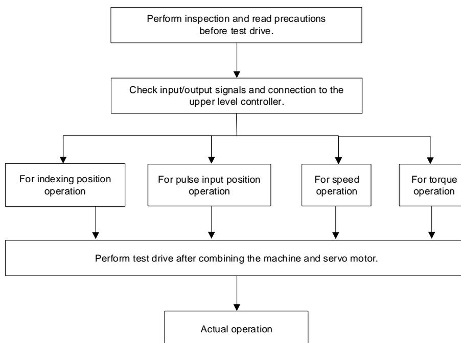
Before a test drive, make sure that wiring between the upper device and servo drive as well as the parameter settings of the servo drive are proper.
