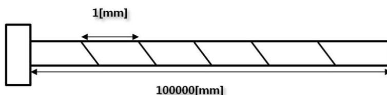
For example, assume that there is a ball screw which moves 1 [mm] for every one full turn of the motor whose encoder has a resolution of 524288 [ppr]. To move the screw by 1 [mm], you have to input 524288 [Pulses] into the servo. If you wish to move it by 27 [mm], addition calculations are necessary and you have to input the complex value of 14155776 [Pulse].
