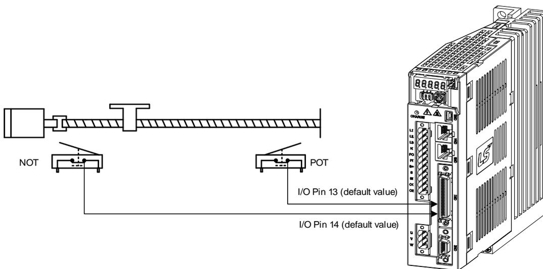
When a positive/negative limit signal is input, the motor stops according to the emergency stop setting (0x2013).
