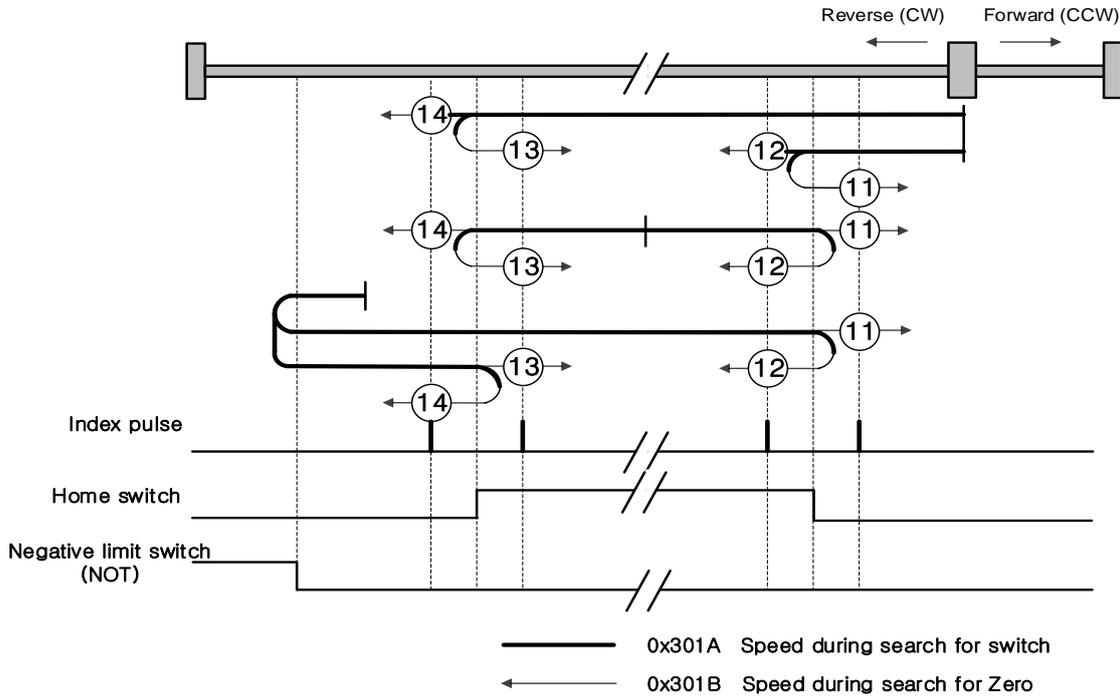
For homing using homing method 14, the velocity profile according to the sequence is as follows. The sequence varies depending on the relationship between the load position and the home switch during homing, which is categorized into three cases as below. For more information, see the details below.
