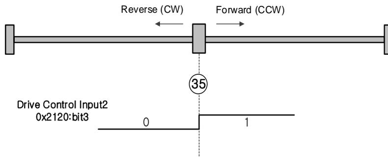
The current position at start of homing operation becomes the home position. This method is used to make the current position the home position according to the demand of the upper level controller.
