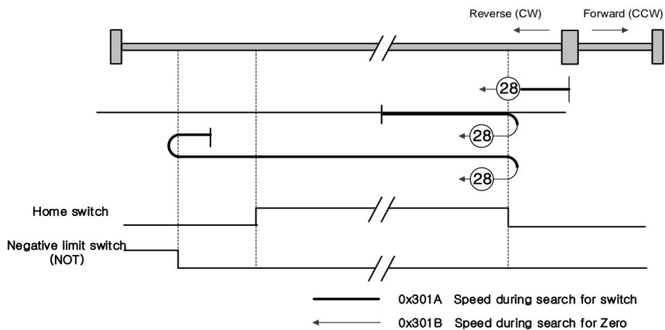
The initial driving direction is reverse (CW), and the point where the negative home switch is turned on becomes the home position.
