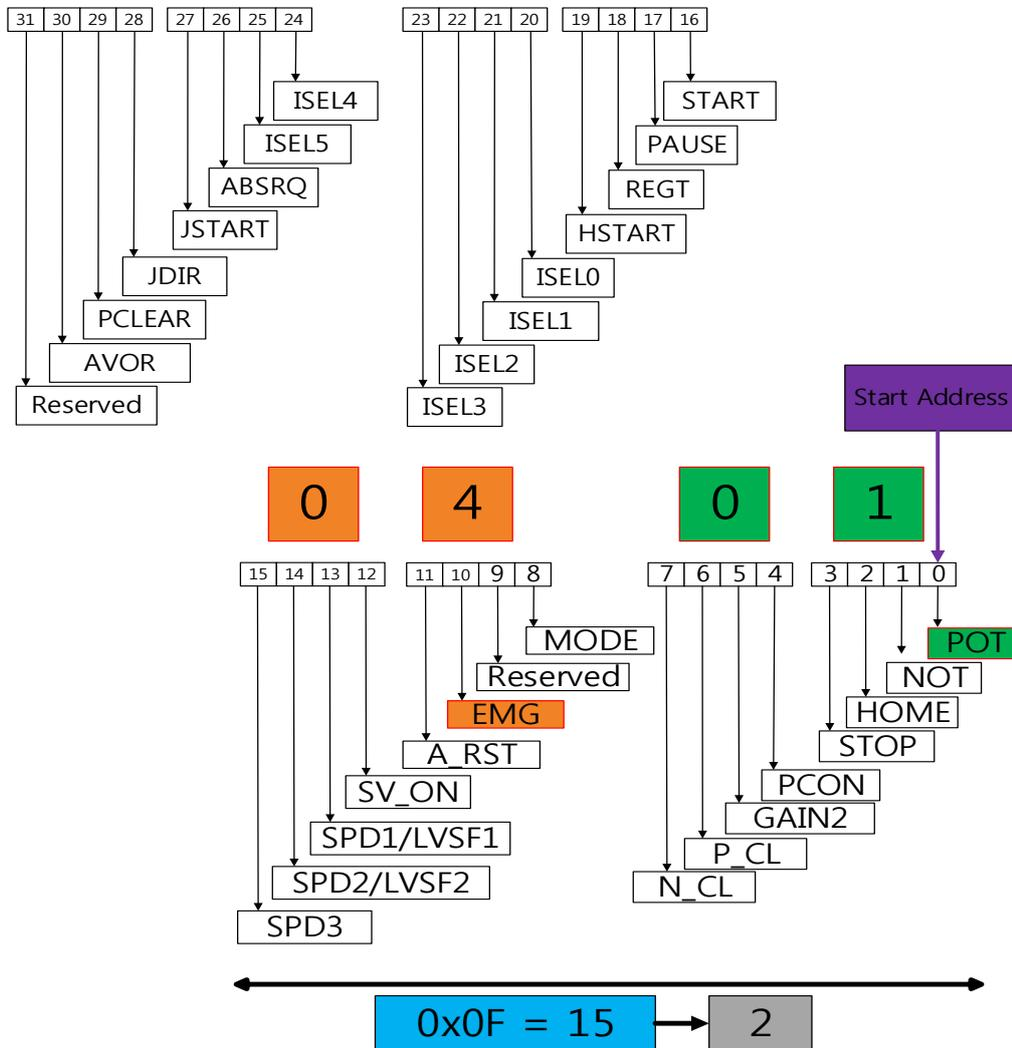
When you assign 15 Quantity Of Outputs while starting from 0x00 for the starting address, you can control the input up to 0x14. As the upper and lower Output Values are swapped, please be careful when you input them. When you input '01 04', for example, they will be swapped into '04 01'. 04 will turn on EMG, the 10th bit, and '01' will turn on POT, the 0th Bit.
