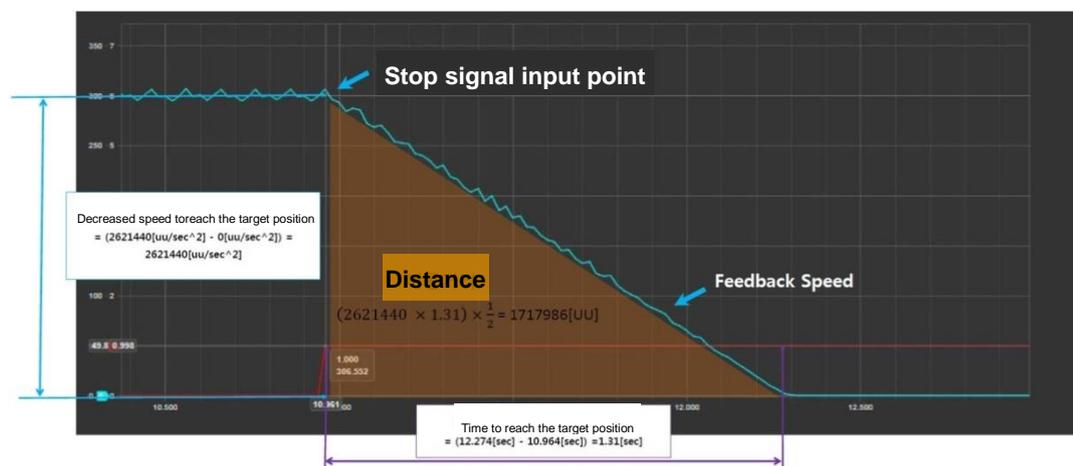
The target position is equal to the area of the distance shown in the figure above. If you want to stop the motor for approximately 2 seconds after inputting STOP signal while the motor is running at 300 rpm in index mode, you can calculate Quick Stop Deceleration as follows.
