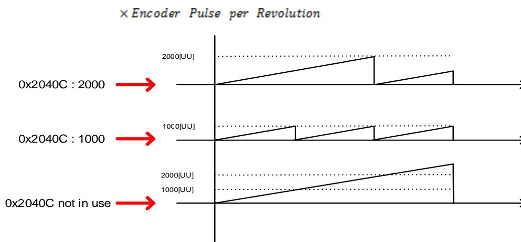
In general, when you do not use the Modulo factor, the current position keeps increasing when the motor rotates in one direction.
