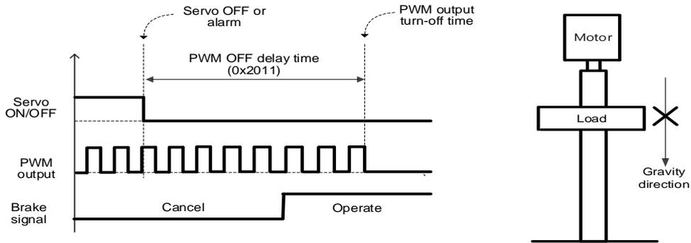
(1) When the brake signal is output before PWM output is turned off
