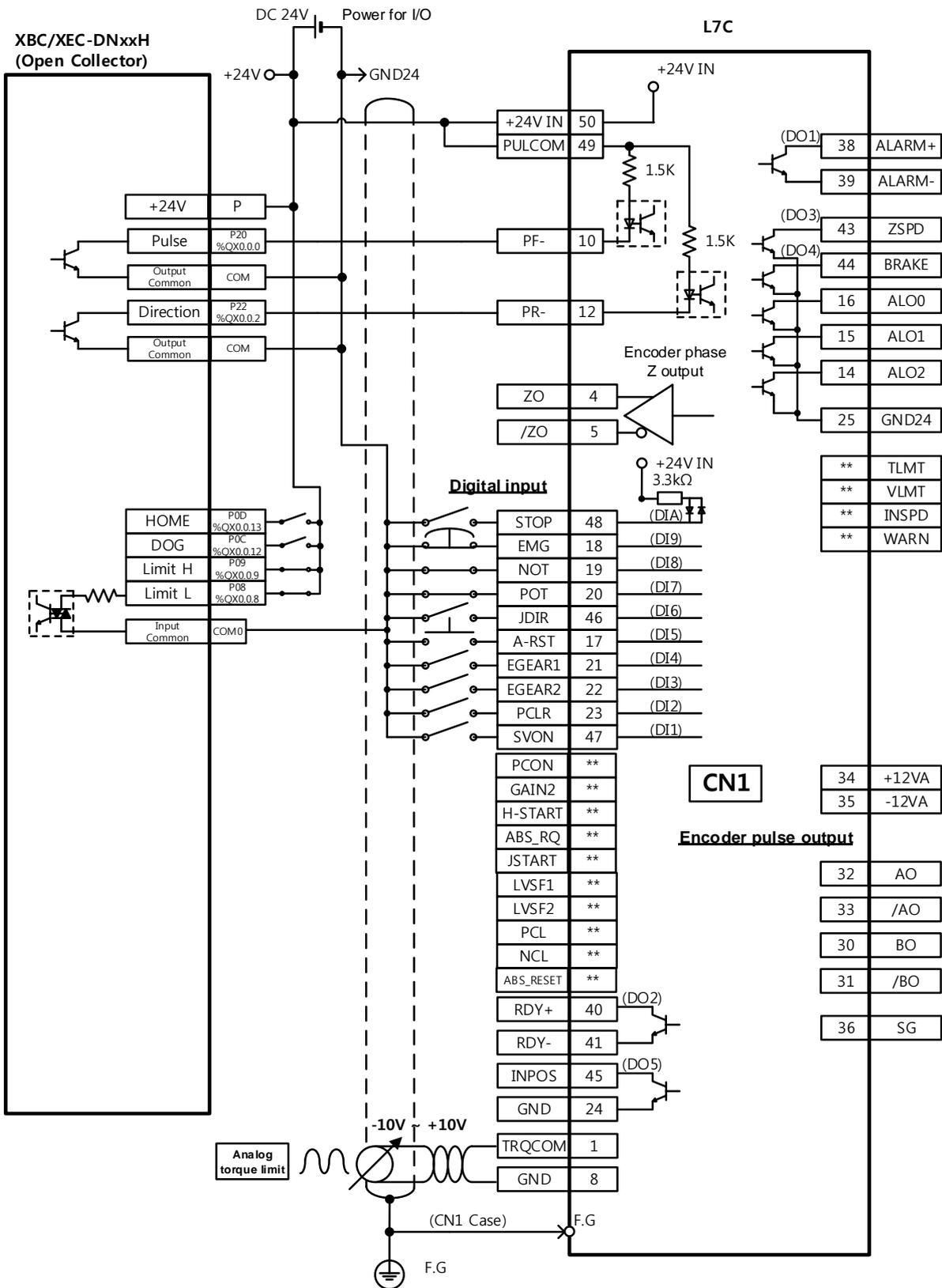
※ This is an example of a wiring diagram for a single shaft. For wiring with 2 shafts, refer to the pin arrangement for the positioning module.
