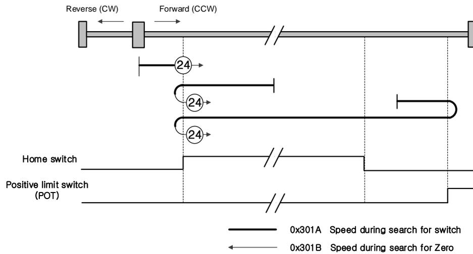
The initial driving direction is forward (CCW), and the point where the positive home switch is turned on becomes the home position.
