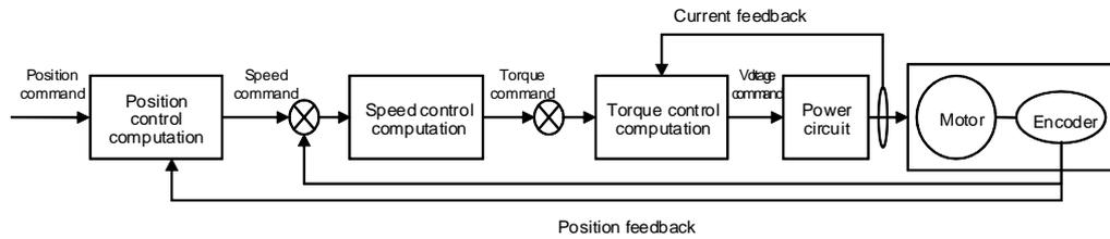
The drive is set to the torque control, velocity control, or position control mode for use, depending on the method of connecting with the upper level controller. This drive has a control structure where position control is located at the outermost part and current control at the innermost, forming a cascade. You can tune the operation according to the purpose by setting gain parameters for the torque controller, velocity controller, and position controller for the drive's operation modes.
