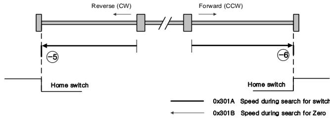
Homing methods -5 and -6 perform homing only by using the stopper. The velocity profile according to sequence is as follows. Homing is stopped when the drive meets the limit switch. For more information, see the details below:
