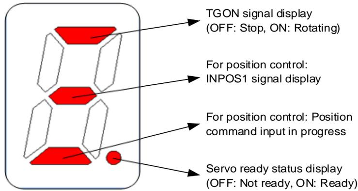
Digit 5 displays the current control mode status and servo on status.
