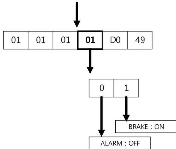
If you set Quantity of Output to 02 for the start address of 0x0020 in the sending protocol, a total of 2 input status values from 0020~0021 are requested. Since Outputs Status Bits of the received protocol is 01, BRAKE is ON and ALARM is OFF.
