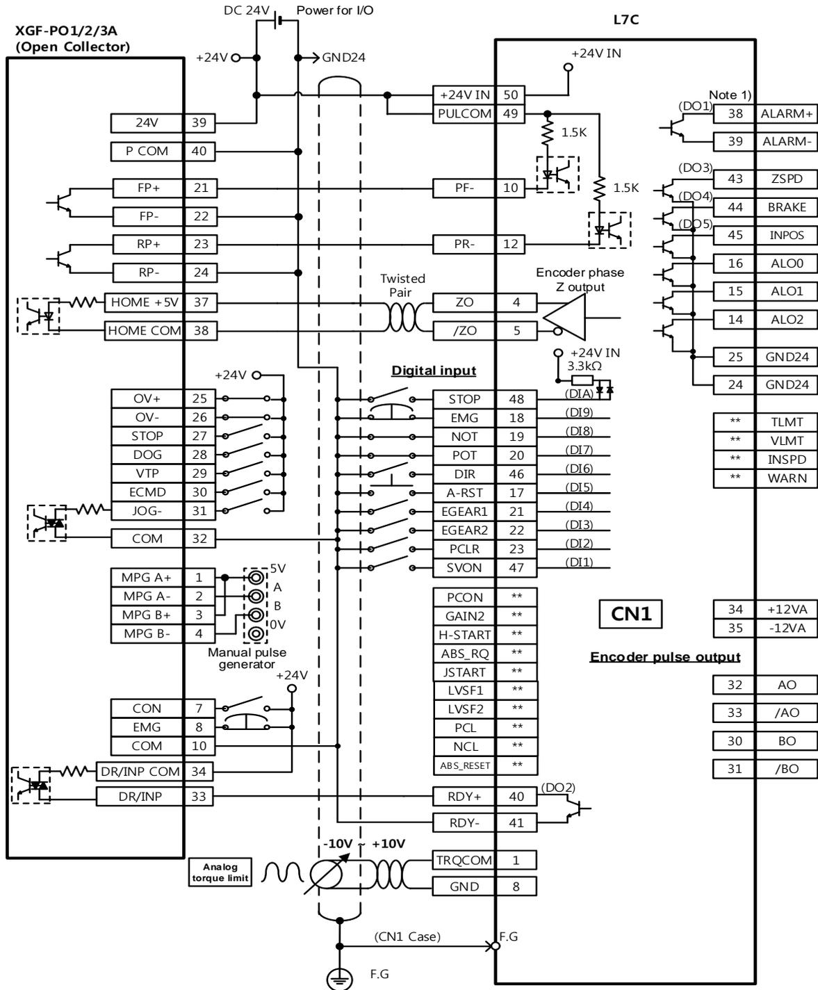
※ This is an example of a wiring diagram for a single shaft. For wiring with 2 or 3 shafts, refer to the pin arrangement for the positioning module.
