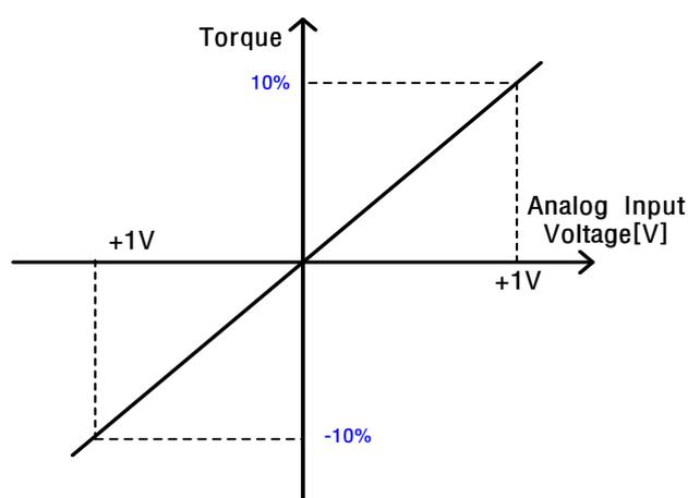
The related object is the 0x2210 analog torque input (Command/limit) scale, which consists of two functions.
