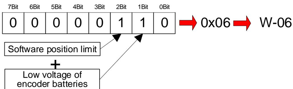
If two warnings occur at the same time, each corresponding bit is set to 1. For example, when a software position limit warning is triggered, the second bit is set. Also, when an encoder battery low voltage warning is triggered, the first bit is set. The two warnings are combined into '0x06,' and you can view the alarm in the display of 'W06' on the segment window.
