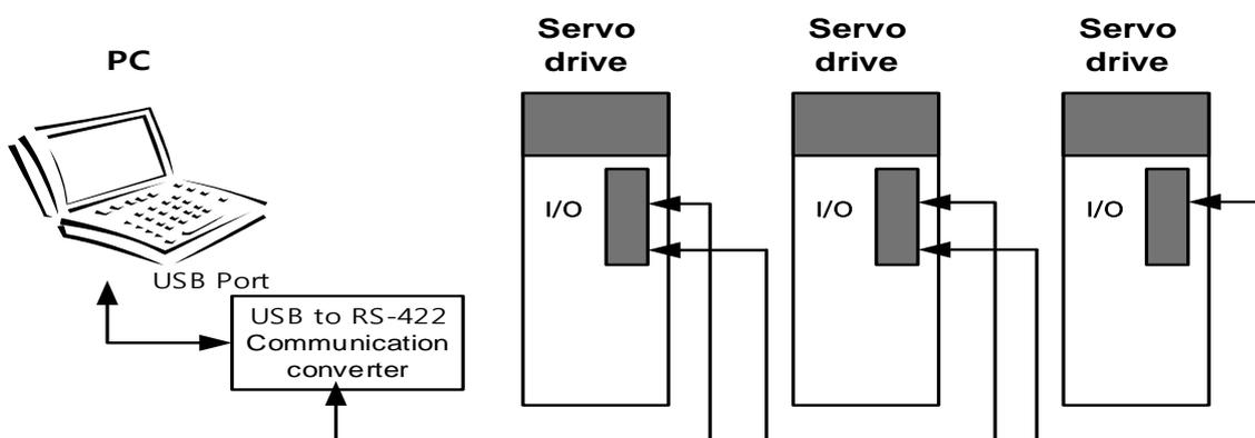
**Note1)** When using a PC as the upper level controller, you have to use the USB-to-RS-422 communication converter.
