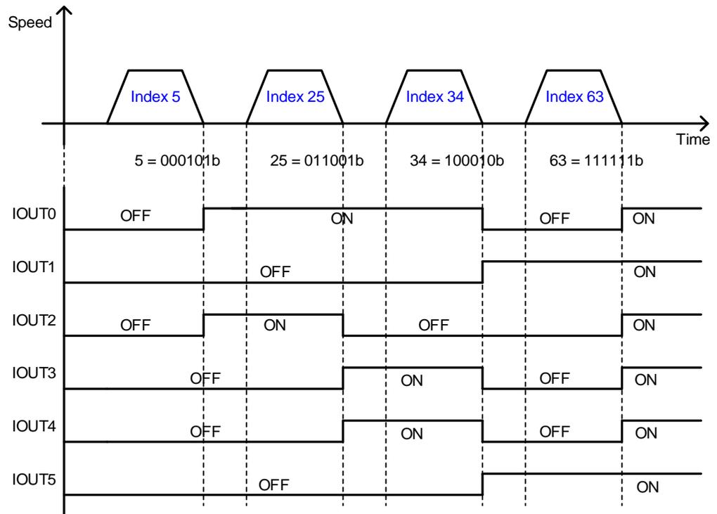
The current index position output signals are initialized when the operation mode is changed or the SVON signal is turned off (Motor free-run state). The initialized output state is identical to the operation status output of the number 0 index, which is why it is advisable to start with Index 1 whenever possible.
