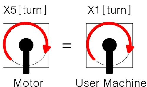
When the machine's apparatus makes 1 [turn], the total pulse required for the machine's 1 [turn] for the installed L7 19 [bit] motor's 5 [turn] is as follows.
