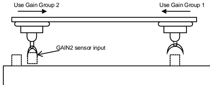
This is one of the gain adjustment functions and is used to switch between Gain Groups 1 and 2. You can reduce the time required for positioning through gain conversion.
