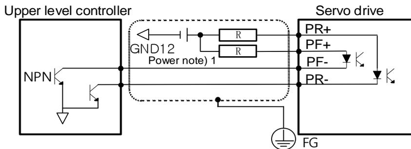
**Note 1)** When using 5[V] power: Resistance  $R = 100\text{-}150\ \Omega$ ,  $1/2\ \text{W}$
