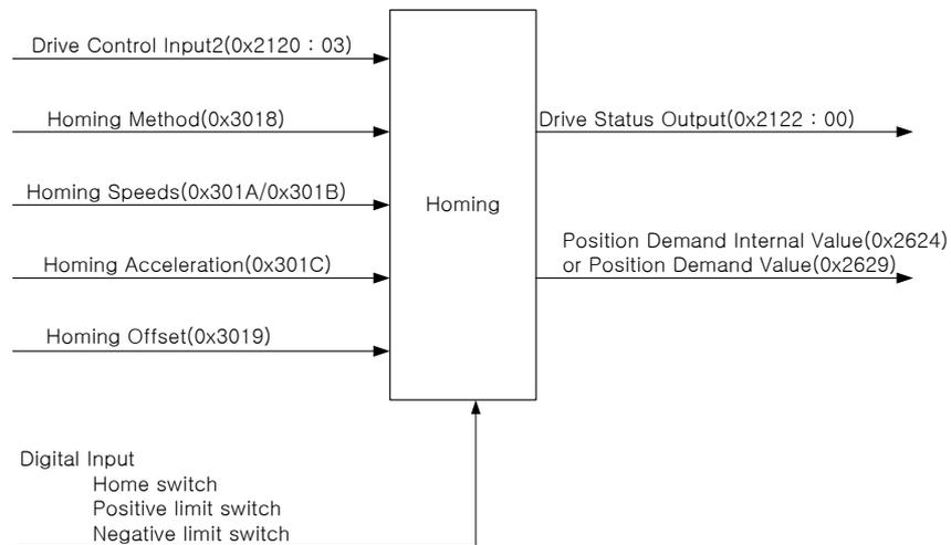
As shown in the figure below, you can set the offset between the home position and the zero position of the machine using the home offset function. The zero position indicates the point whose Position Actual Value (0x262A) is zero (0).
