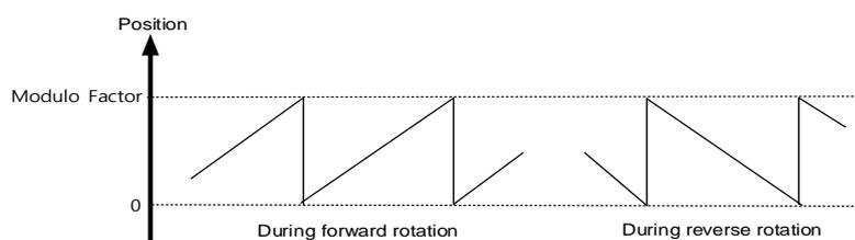
You must set the control mode (0x3000) to the rotary coordinate system to enable the below 5 PTP position controls. Here, the Modulo Factor setting must be proper.
