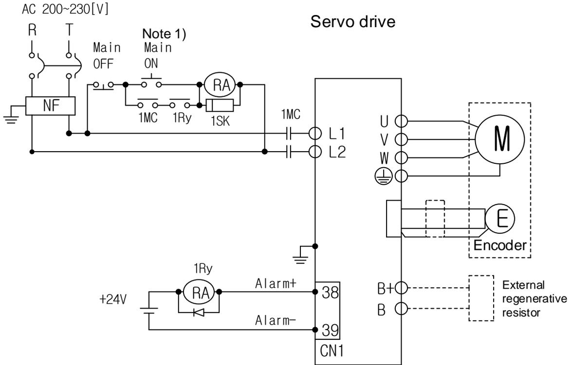
**Note1)** About 1~2 seconds are required from main power supply to alarm signal output. Press the main power on switch and hold it for at least 2 seconds.
