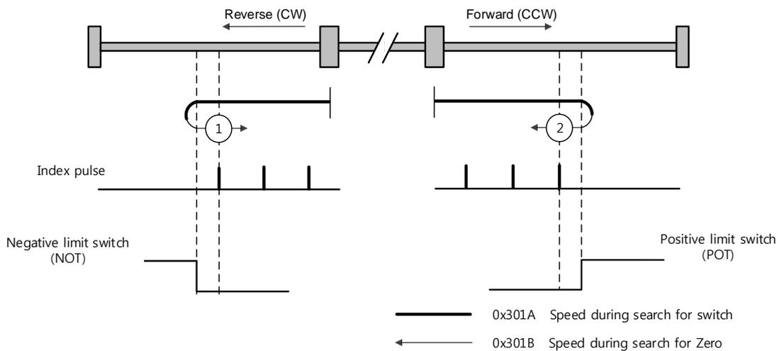
For homing using the homing method 1, the velocity profile according to the sequence is as follows. Refer to the description below.
