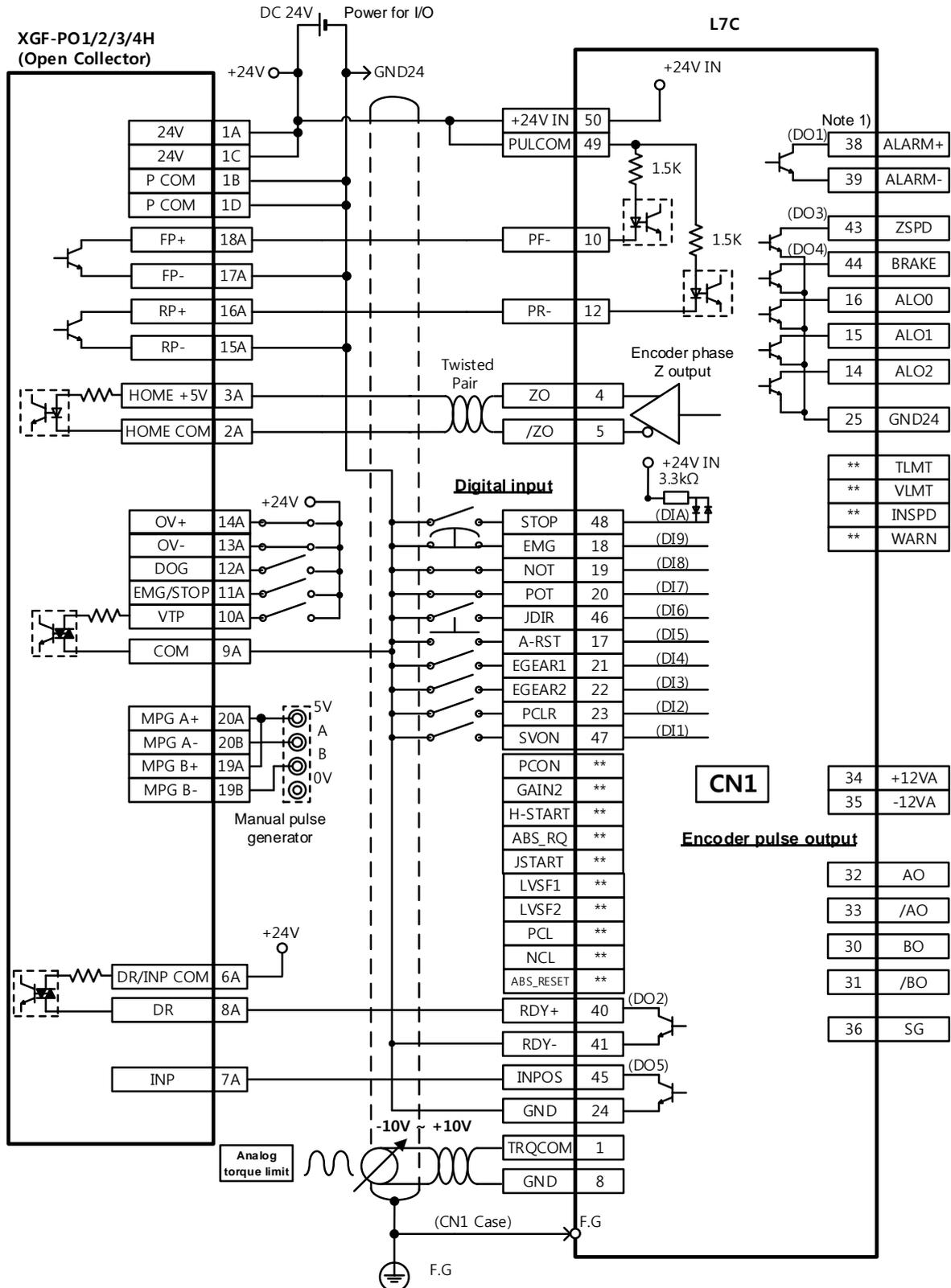
※ This is an example of a wiring diagram for a single shaft. For wiring with 2, 3, or 4 shafts, refer to the pin arrangement for the positioning module.
