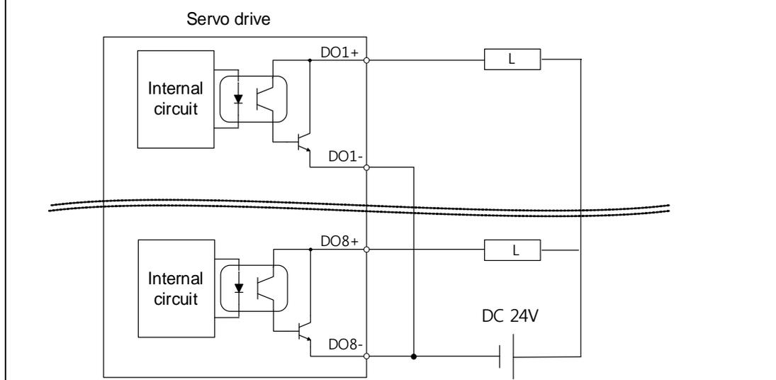
**Note 1)** DO1 and DO2 outputs use separated GND24 terminals, and DO3~DO8 outputs use a common GND24 for DOCOM.
