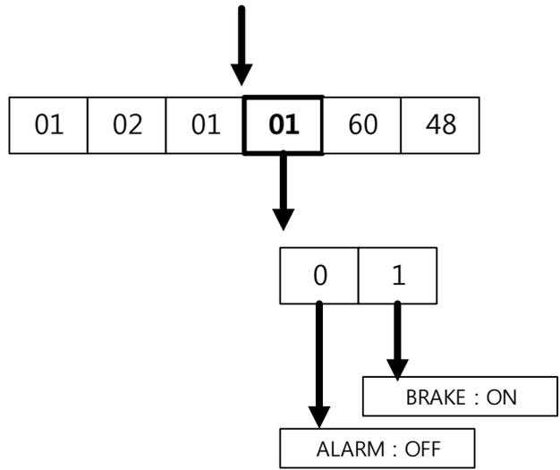
2) Example of parameter reading for 0x0020~0x0022
