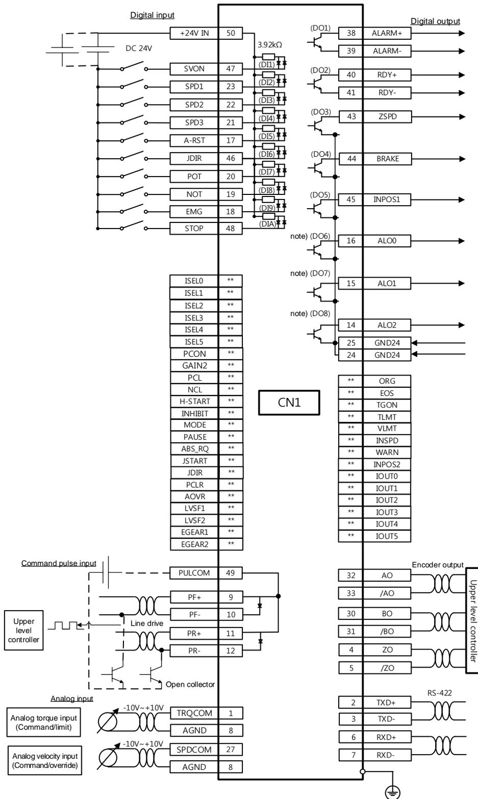
Note 1) Input signals DI1~DI10 and output signals DO1~DO8 are factory default signals. Note before use that DO6~DO8 are locked output ports for which assignment is not possible.
