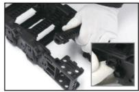
Assembly a specified frame in M.FEB and F.FEB. (Hinge is inserted into RH direction of FEB) Insert Frame pin into connected frame and side of
