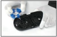
Insert BR Unit into each Side Band (Side Band is divided into right and left side according to the direction.)
