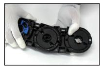
Continue to insert BR Unit into Side Band as you want to make it Assemble Side Band which is inserted BR Unit as above.
