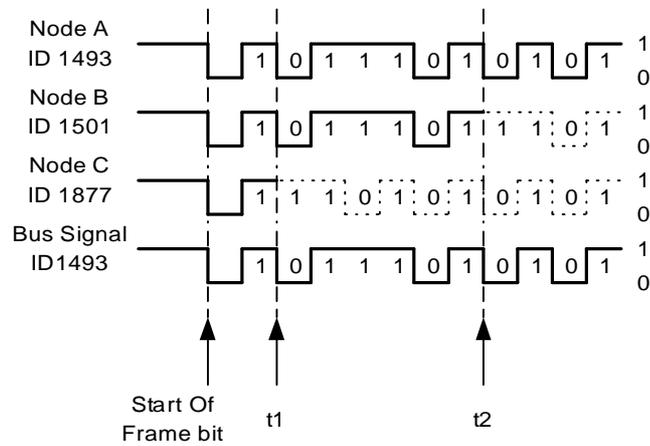
After the start of frame bit, each node starts to transmit its message identifier. At time  $t_1$ , node C transmits a recessive bit (logic 1). Nodes A and B transmit dominant bits (logic 0), so the bus level goes to logic 0. Node C sees that the data it transmitted is not reflected on the bus data, and therefore other nodes have a higher message priority. It will stop transmitting, and will wait for the next arbitration cycle before trying again.
