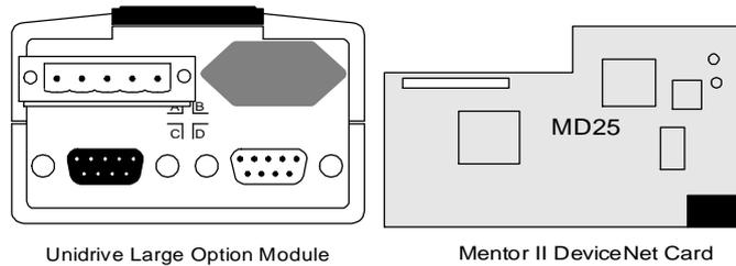
The DeviceNet connector provides power and also communications. Cables should be wired according to the following table. (Pin 1 is the left-most pin on the connector.)
