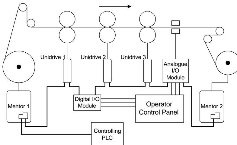
Unidrive 3 is the master Drive in the system. This receives the master speed reference from the PLC, and transmits the post-ramp speed reference back to the PLC. The post-ramp speed reference is scaled, and becomes the line speed reference for the Mentor II Drives.
