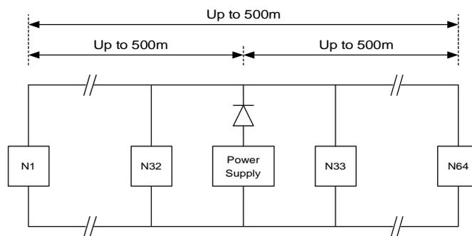
For detailed instructions on determining power supply requirements and configuration, refer to "DeviceNet Installation" from Rockwell Automation, Publication 1485-6.7.1.
