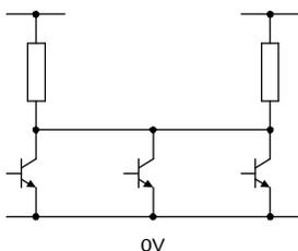
With CAN-based networks, logic 0 on the network is “dominant”, while logic 1 is “recessive”. The “wired AND” nature of CAN means that when the bus is at logic 1, it is not actually being held at logic 1 by any particular node. Any node can therefore take the bus to logic 0, without damaging any other nodes. Hence the terms “dominant” and recessive.
