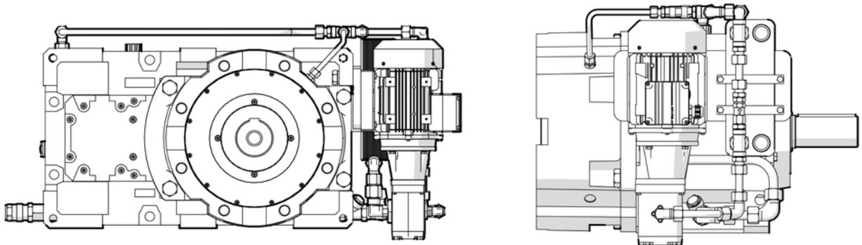
The plate exchanger is a water/oil cooling system, which can be fed by a motor pump as shown, or by a mechanical pump.
