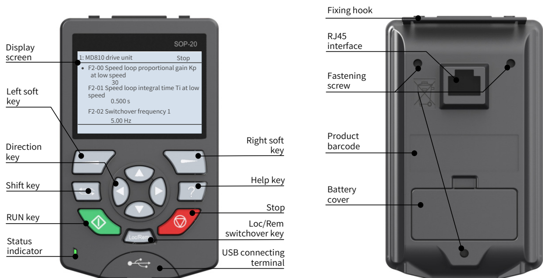
Figure 4-5 Appearance of external LCD operating panel
