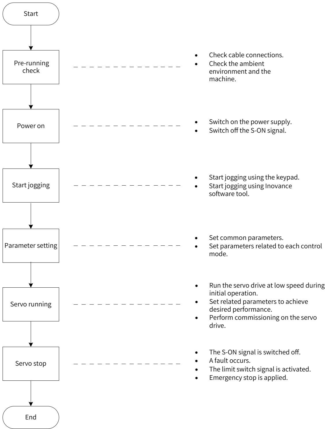
Figure 5-1 Flowchart for setting the servo drive
