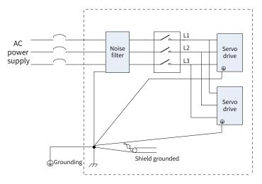
Figure 3-30 Grounding cable of the noise filter
