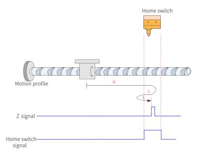
Figure 7-18 HW signal inactive at start
