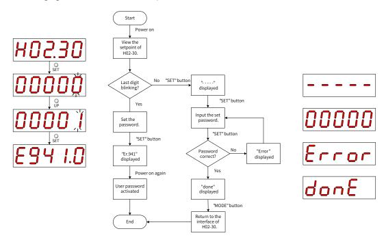
Figure 4-6 Procedure for user password setting
