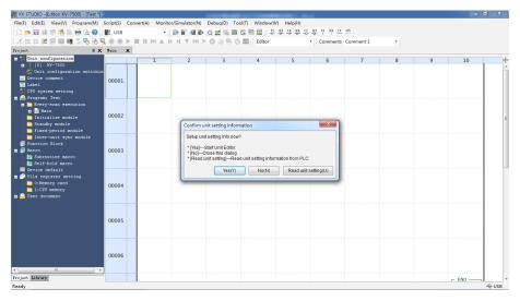
Click **Read unit setting** when the physical PLC unit is connected properly and able to communicate with the software tool. The software tool obtains unit settings automatically according to the physical connection.
