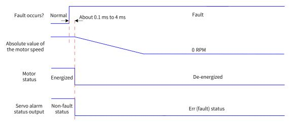
Figure 5-11 Timing diagram of "coast to stop, keeping de-energized status" at No. 1 fault
