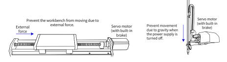
Figure 5-2 Application of the motor brake
