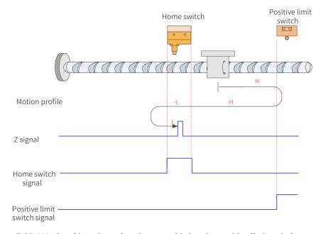
Figure 7-28 HW signal inactive at homing start, hitting the positive limit switch
