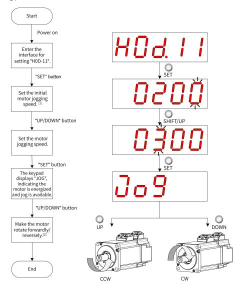
Figure 4-7 Procedure for setting the jog function
