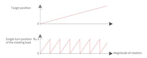
The variation law of the target position and the single-turn position of the rotating load during reverse running is shown as follows.
