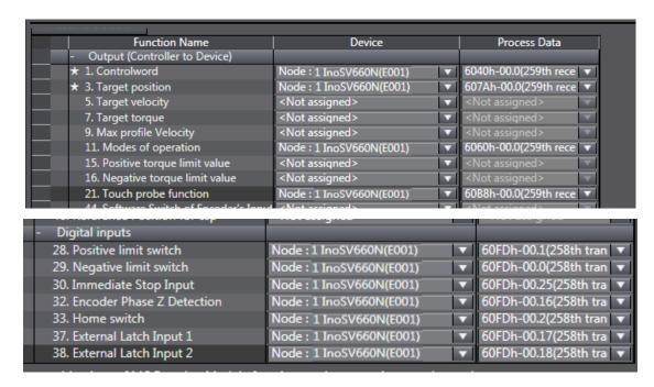
60FDh must be mapped to objects by bit. The mapping must be consistent with that in the Omron controller. SV660N only supports the positive/negative limit, home function, and touch probe function.
