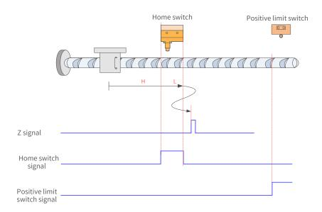
Figure 7-33 HW signal inactive at start, not hitting the positive limit switch
