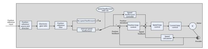
Figure 6-8 Operating process for speed feedforward control
