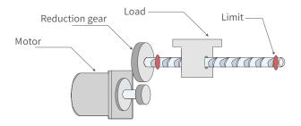
Figure 7-86 Application of the linear mode
