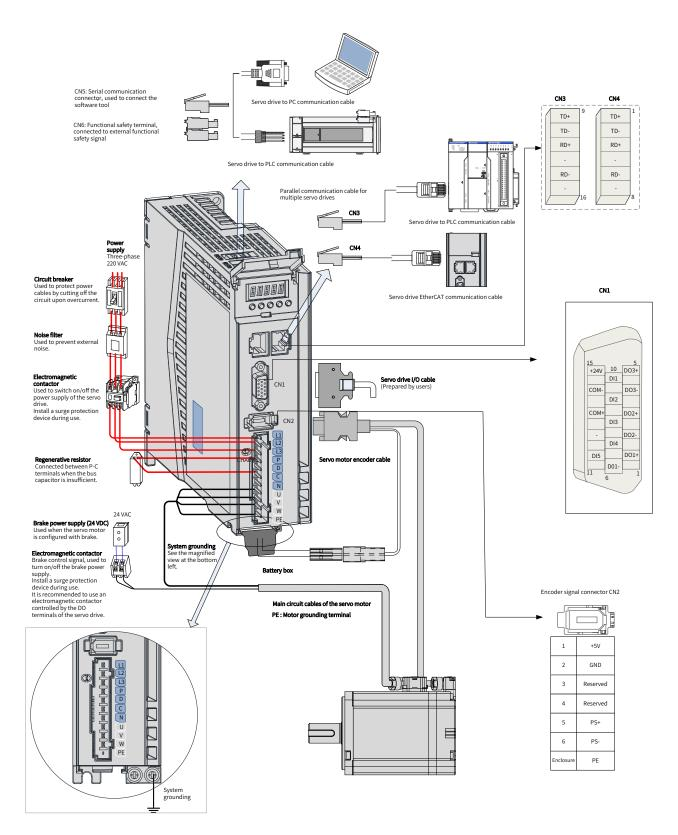
Figure 1-14 Wiring of three-phase 220 V systems
