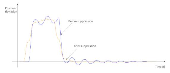
Figure 6-16 Effect of low-frequency resonance suppression
