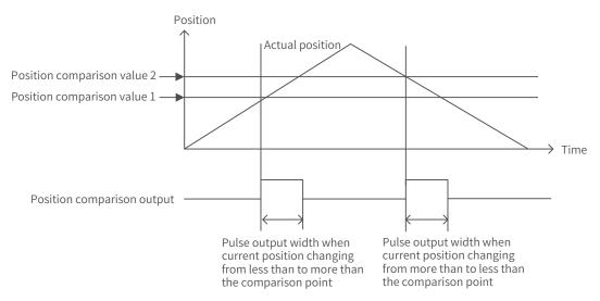
When the attribute of the comparison point is set to 1 (Output DO active signal if current position changes from "less than" to "more than" the comparison point), the DO outputs the position comparison signal when the axis position changes from "less than" to "more than" the comparison point position.
