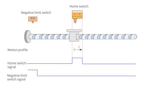
Figure 7-74 HW signal active at start
