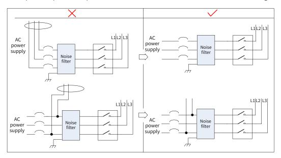
Figure 3-27 Separate routing of input and output cables
