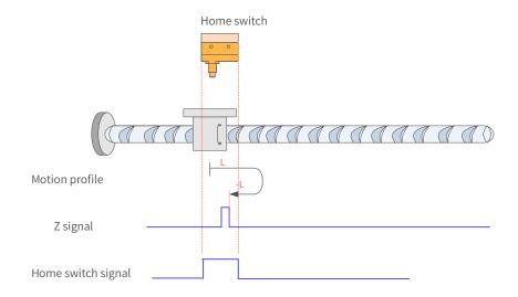
Figure 7-23 HW signal active at start
