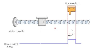
Figure 7-52 HW signal inactive at start
