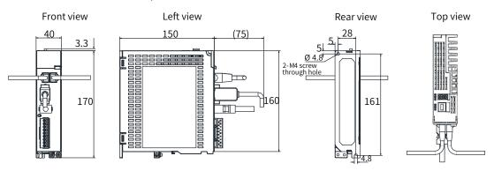
Fixing screw: 2-M4 Recommended tightneing torque: 1.2 N·M
