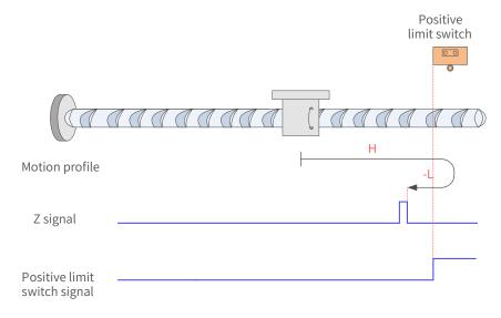
Figure 7-14 P-OT signal inactive at start
