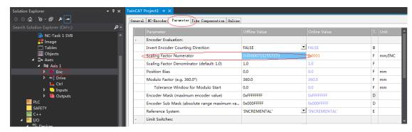
■ **Scaling factor Numerator**: Indicates the distance corresponding to the encoder pulses per position feedback.
