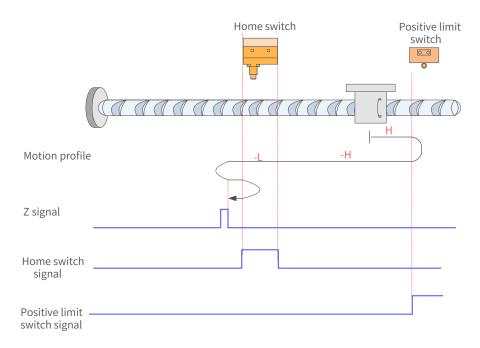
Figure 7-25 HW signal inactive at homing start, hitting the positive limit switch
