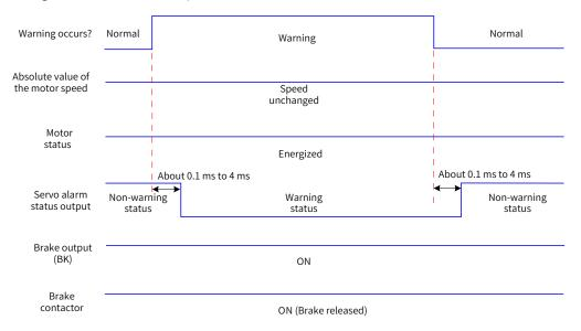
Figure 5-19 Timing diagram at warnings that do not cause stop
