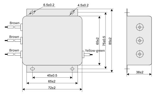
Figure 12-7 Dimensions of the safety capacitance box
