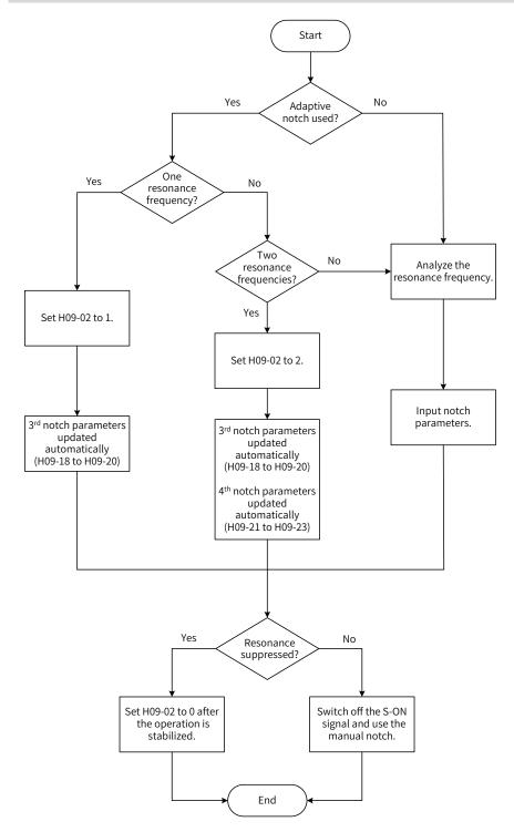
Figure 6-12 Procedure for using the notch
