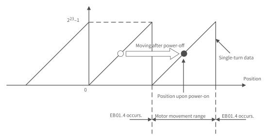
c) Note: When the power supply is switched on near the motor movement range limits, EB01.4 (Target position beyond the limit) may easily occur.
