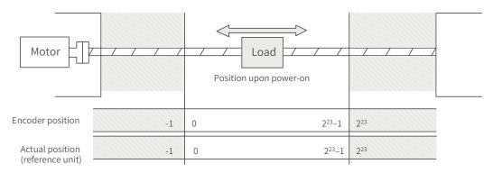
When the gear ratio is 1:1, and 607Ch is set to 10000, the position range is as shown in the following diagram.
