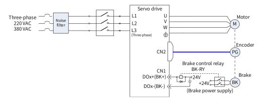
Figure 3-21 Wiring of the brake
