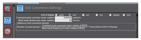
Select **Unit of display** based on the actual running unit when setting the gear ratio. All the position-type parameters in the host controller will be displayed in this unit.
