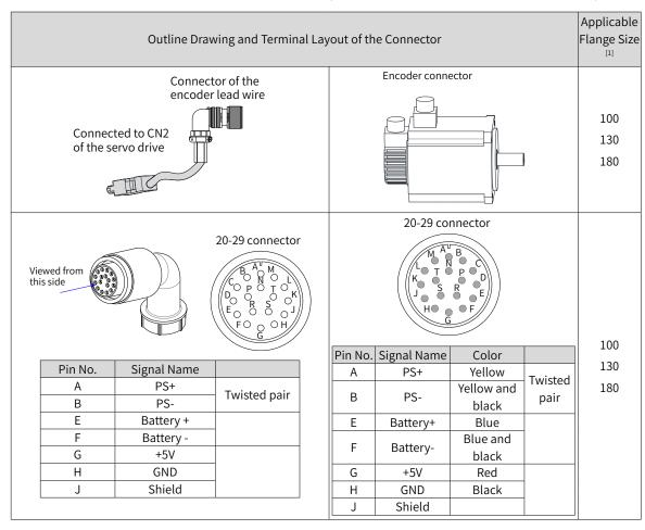
Table 3-20 Absolute encoder cable connector (MIL-DTL-5015 series 3108E20-29S connector)
