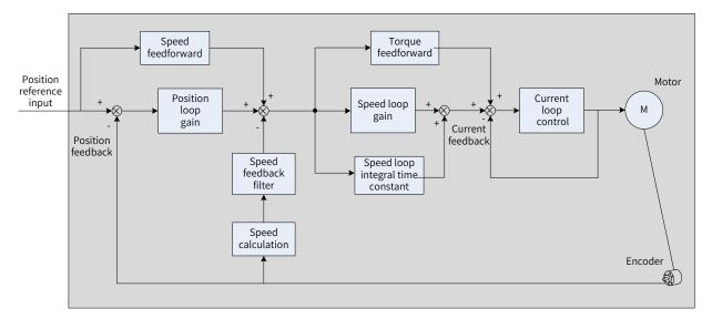
Figure 6-5 Basic control diagram
