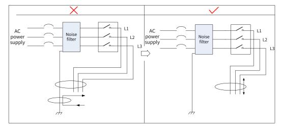
Figure 3-28 Separate routing of the grounding cable and the power output cable
