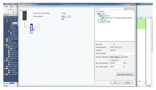
After adding the axes, click **OK**. The following dialogue box opens, asking you whether to set up coordinate transformation.
