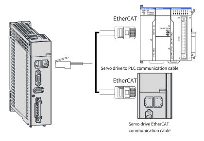
Figure 3-23 Wiring of communication cables
