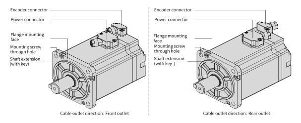
Figure 1-8 Components of MS1 series terminal-type motors
