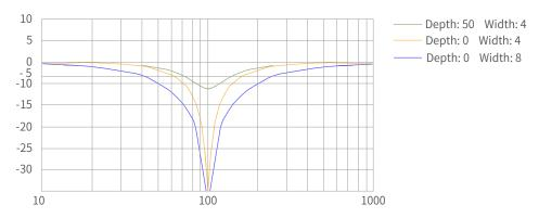
Figure 6-13 Notch frequency characteristics
