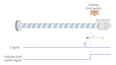
Figure 7-15 P-OT signal active at start
