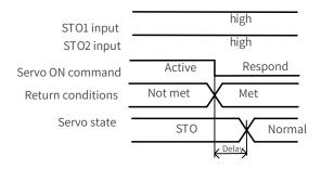
Figure 12-12 Return condition of S-ON/RUN command
