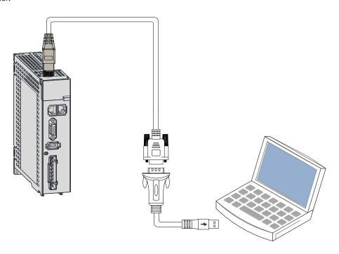
Figure 3-25 Serial-to-USB conversion
