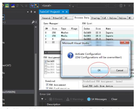
c) After clicking **OK**, the device enters OP status as shown in the **Online** interface. The 3rd LED on the keypad displays the value 8, and the keypad displays \_88RY.
