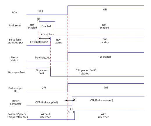
Figure 5-20 Timing diagram of fault reset
