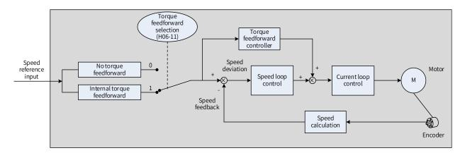
Figure 6-9 Operating process for torque feedforward control
