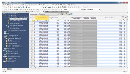
2. Move the mouse to the point parameter, such as No.1-Axis1, and wait until the mouse icon to change from an arrow to a small hand. Then drag towards the program edit interface with mouse right button, and the following shortcut pops out.
