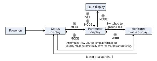
Figure 4-2 Switchover between different display modes
