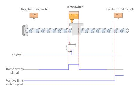
Figure 7-29 HW signal active at start
