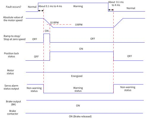
Figure 5-18 Timing diagram for warnings that cause stop
