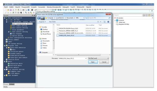
You can add the axes needed through dragging or double-clicking. Select the corresponding axis, and set critical information such a **Encoder resolutuion**, **Max. motor speed**, and **Max. motor torque** for this axis. You can add PDO setting in detailed setting of the slave.
