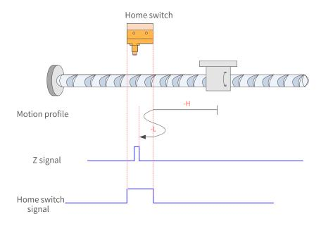
Figure 7-22 HW signal inactive at start
