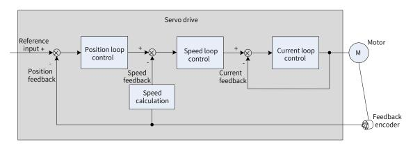
Figure 7-1 Structure of a basic servo system
