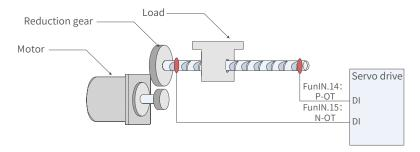
Figure 7-85 Installation of limit switches
