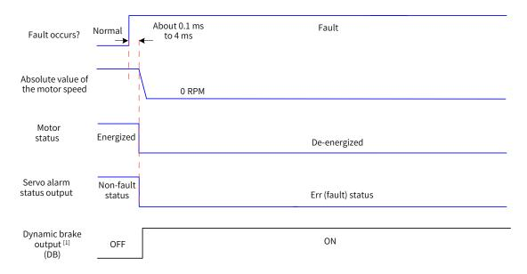
Figure 5-15 Timing diagram of "Coast to stop, keeping de-energized state" at No. 2 fault (without brake)
