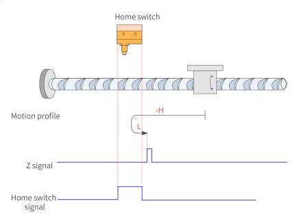
Figure 7-20 HW signal inactive at start
