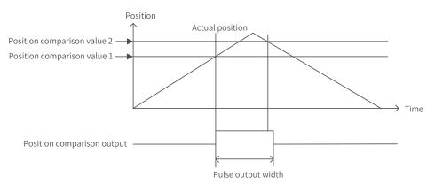
• Only one pulse will be output when the stop position is the same with the target value of position comparison, as shown in the following figure.
