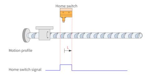
Figure 7-57 HW signal active at start
