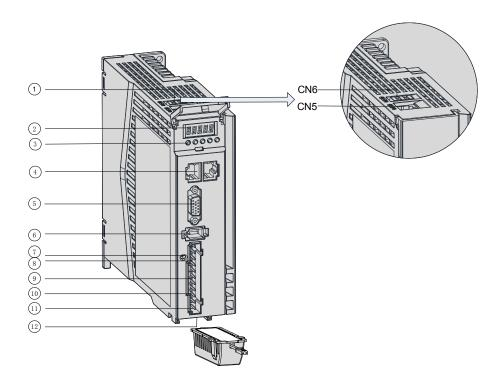
Figure 1-4 Layout of servo drives in size B
