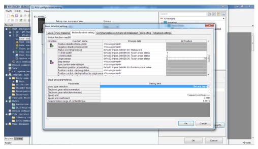
Set the restriction parameters for homing in **Axis control setting** > **Origin return**. The following homing methods are available. For detailed trajectories, see KEYENCE instruction manual for positioning/motion control unit KV-XH16EC.
