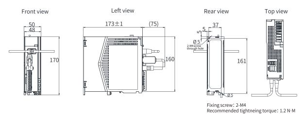
Figure 2-2 Outline dimensions of size B (unit: mm)
