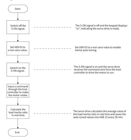
Figure 6-4 Procedure for online inertia auto-tuning
