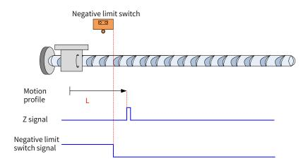
Figure 7-13 N-OT signal active at start
