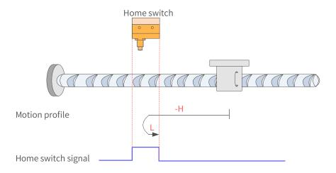
Figure 7-56 HW signal inactive at start
