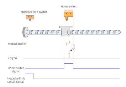
Figure 7-41 HW signal active at start
