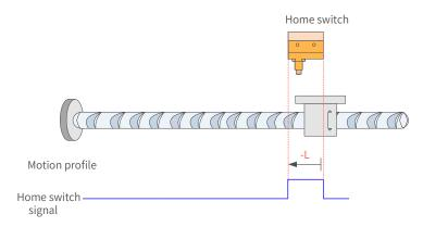
Figure 7-53 HW signal active at start
