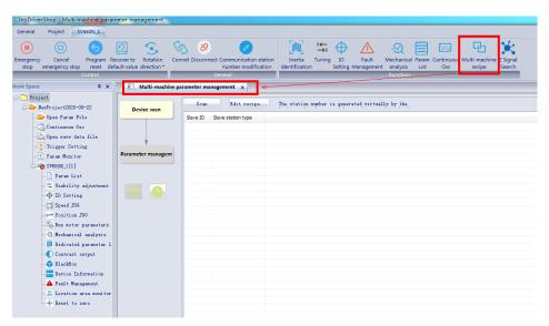
2) Scanning: Click the **Scan** button, and all the EtherCAT slaves cascaded will be scanned and displayed. The scanning time is directly proportional to the number of cascaded slaves, so you may wait a few minutes in case of large numebers of cascaded slaves. (Non-Inovance slaves are displayed as "Non-Inovance device".)
