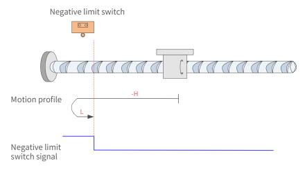
Figure 7-48 N-OT signal inactive at start
