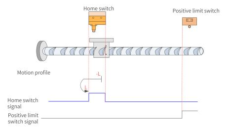
Figure 7-65 HW signal active at start
