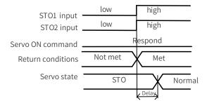
Figure 12-13 Return condition of external STO request state
