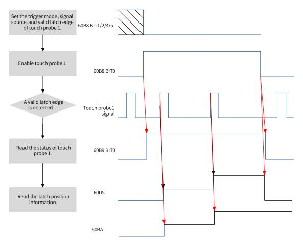
Figure 7-84 Operaing procedure of touch probe function
