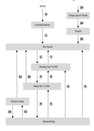
Figure 7-2 CiA402 state machine switchover
