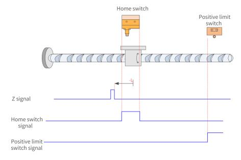
Figure 7-26 HW signal active at start
