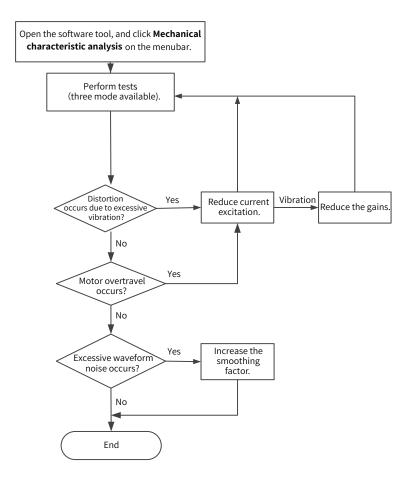
Figure 6-17 Operating procedure for mechanical characteristic analysis
