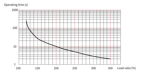
Figure 1-11 Motor overload curve
