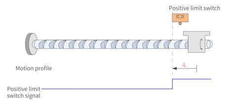
Figure 7-51 P-OT signal active at start
