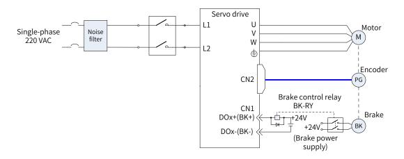
Figure 5-3 Wiring of the motor brake
