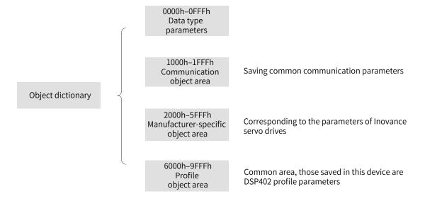
Figure 8-1 Structure of CANopen object dictionary
