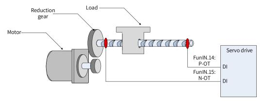
Figure 5-21 Installation of limit switches
