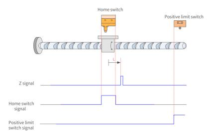
Figure 7-35 HW signal active at start
