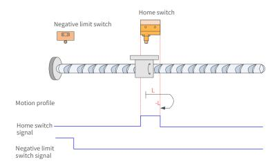
Figure 7-77 HW signal active at start
