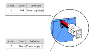
Figure 3-18 Lead wires of the absolute encoder battery
