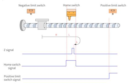
Figure 7-30  $\,$  HW signal inactive at start, not hitting the positive limit switch
