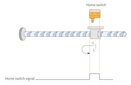
Figure 7-55 HW signal active at start
