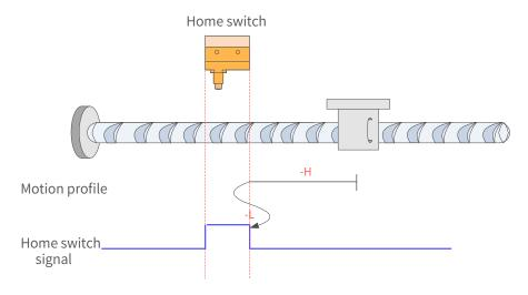
Figure 7-58 HW signal inactive at start
