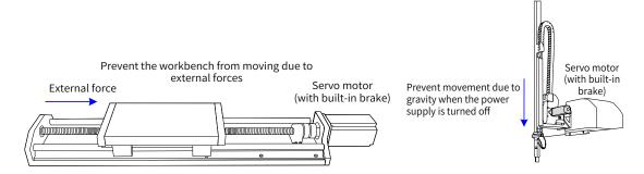
Figure 3-20 Application of the brake
