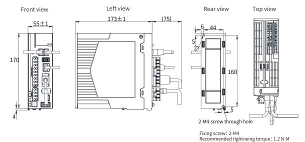
Figure 2-3 Outline dimensions of size C (unit: mm)
