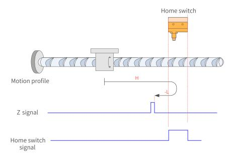
Figure 7-16 HW signal inactive at start
