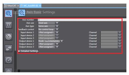
**Axis number**: Represents the Ethernet communication station No. of the servo drive, which is also the value of H0E-21.
