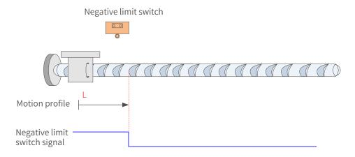
Figure 7-49 N-OT signal active at start
