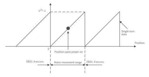
b) To change the motor movement range, turn off the power supply at the position shown in the preceding figure, and turn on the power supply again after moving the motor to the position shown in the following figure.
