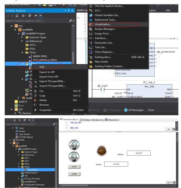
8) Adding the HMI interface to control the servo drive through the HMI interface
