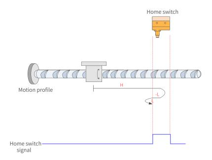
Figure 7-54 HW signal inactive at start
