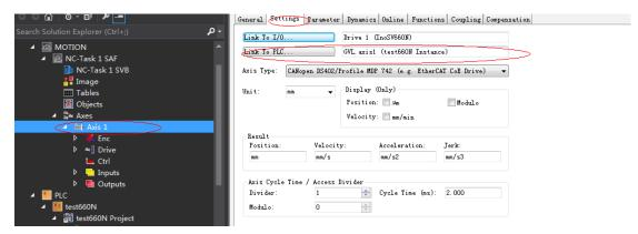
f) Compile the program. If there is not fault, activate the configuration and log onto the PLC.
