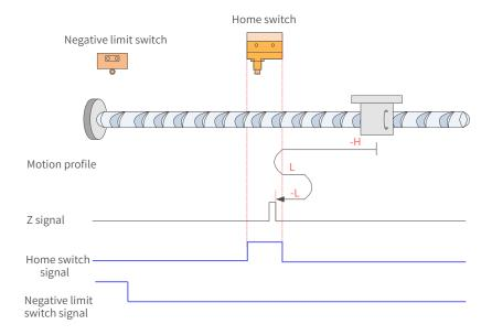
Figure 7-39 HW signal inactive at start, not hitting the negative limit switch
