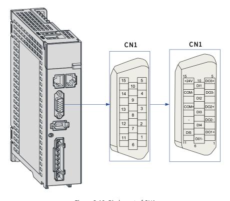
Figure 3-19 Pin layout of CN1
