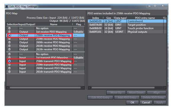
Modify the PDO mapping object through **Add PDO Entry** and **Delete PDO Entry**. The frequently used mapping parameters are shown below.
