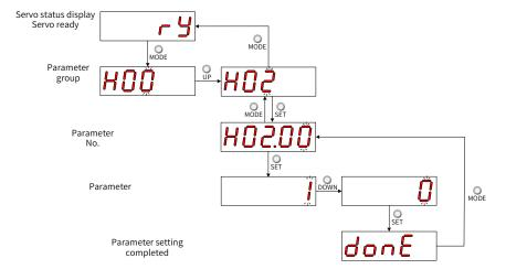
Figure 4-5 Procedure for parameter setting
