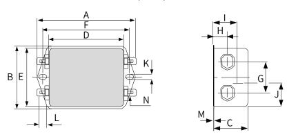
Figure 12-4 Dimensions of FN2080 series filters (1–16 A) (unit: mm)
