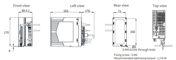
Figure 2-4 Outline dimensions of size D (unit: mm)
