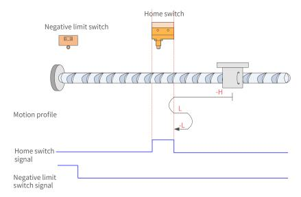
Figure 7-75 HW signal inactive at start, not hitting the negative limit switch
