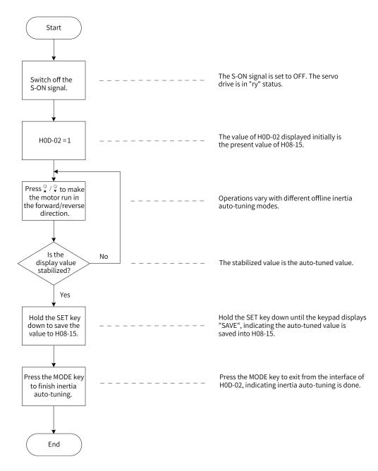
Figure 6-3 Procedure for offline inertia auto-tuning
