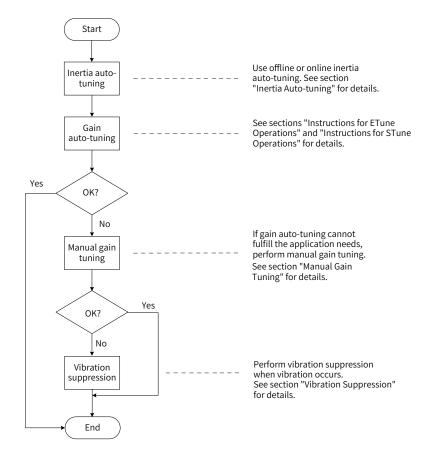
Figure 6-2 General procedure for gain tuning
