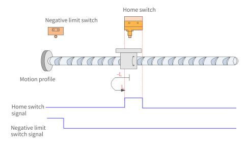
Figure 7-80 HW signal active at start
