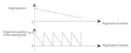
When the motor works in the absolute rotation mode and the servo drive operates in the HM mode, the setting range of the home offset is 0 to  $(R_M-1)$ . If the home offset is set to a value outside this range, the servo drive reports EE09.1 (Home setting error).
