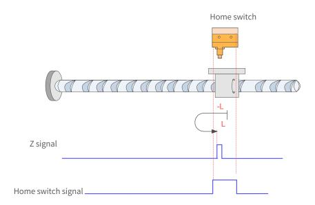
Figure 7-19 HW signal active at start
