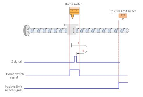
Figure 7-32 HW signal active at start
