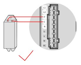
Figure 3-9 Connection of the external regenerative resistor
