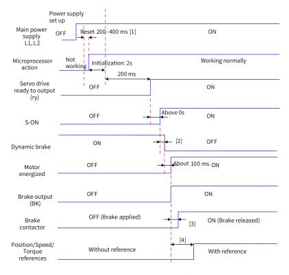
Figure 5-10 Power-on timing diagram
