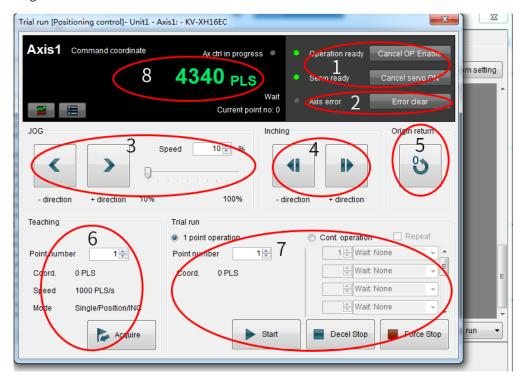
OP enable/Servo ON: Unrelated to the status of the ladder diagram program. OP enable and Servo
