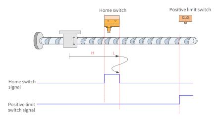
Figure 7-69 HW signal inactive at start, not hitting the positive limit switch
