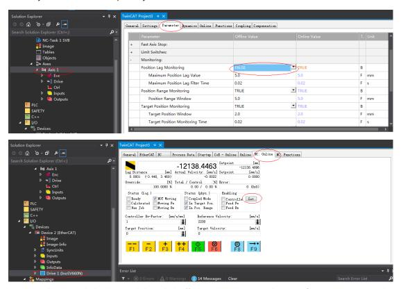
Click **Set** to display a dialog box and then click **All** to enable the servo drive. Perform jogging through F1 to F4. The jog speed is set as follows.
