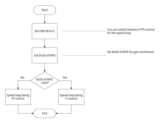
Figure 6-6 Gain switchover flowchart (H08-08 = 0)
