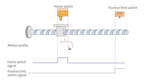
Figure 7-68 HW signal active at start
