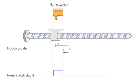
Figure 7-59 HW signal active at start
