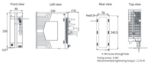
Figure 2-5 Outline dimensions of size E (unit: mm)
