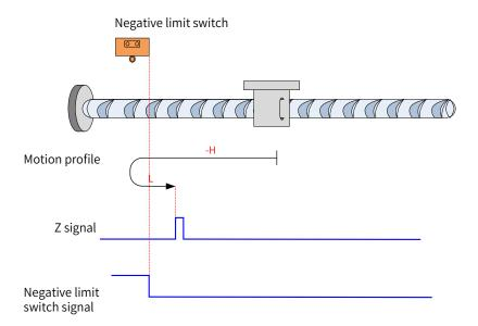
Figure 7-12 N-OT signal inactive at start
