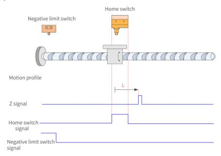
Figure 7-38 HW signal active at start
