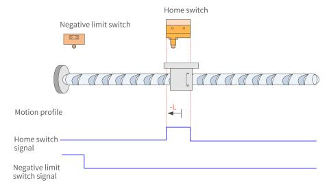
Figure 7-83 HW signal active at start
