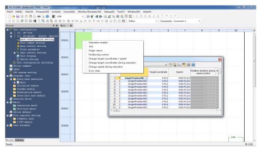
Select the function needed, such as **Operation enable**, click it to generate a DEMO program automatically. Then designate the part in red as the relay needed. After these actions are done, this function is done compiling.
