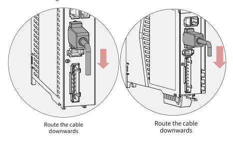
Figure 2-7 Routing direction
