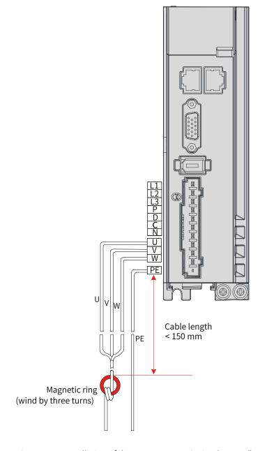
Figure 12-8 Installation of the output magnetic ring (external)
