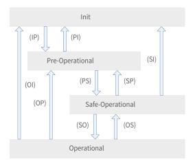
Figure 9-3 EtherCAT state machine
