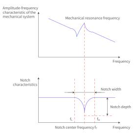
Figure 6-11 Operating principle of the notch
