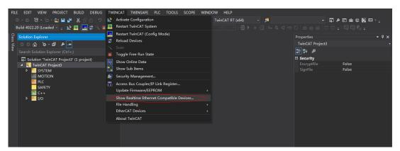
Open **Show Real Time Ethernet Compatible Devices...** in the menu shown in the preceding figure to display the following dialog box. Select local connection under **Incompatible devices**, and click **Install**. After installation is done, the network adapter installed will be displayed under **Installed and ready to use devices(realtime capable)**.
