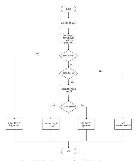
Figure 6-7 Gain switchover flowchart (H08-08 = 1)
