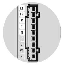
Figure 3-5 Main circuit terminal pin layout of servo drives in size A
