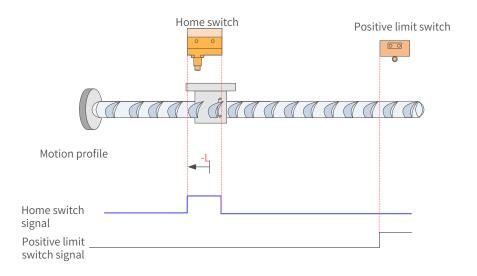
Figure 7-62 HW signal active at start
