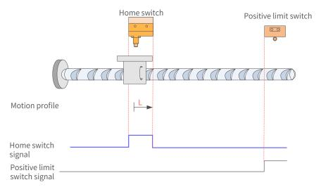
Figure 7-71 HW signal active at start
