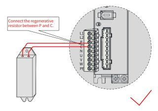
Figure 5-8 Connection of an extenal regenerative resistor
