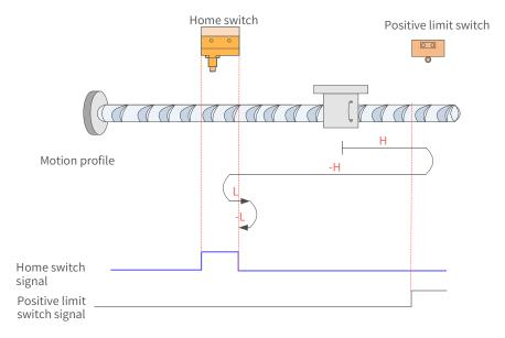
Figure 7-67 HW signal inactive at start, hitting the positive limit switch
