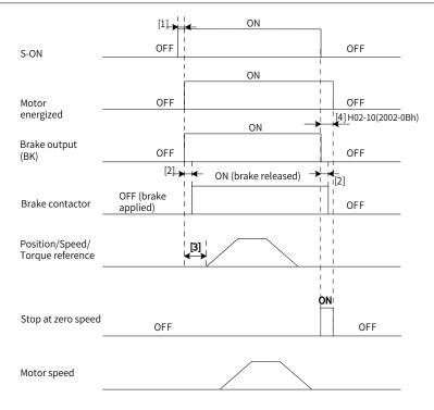
Figure 5-4 Brake time sequence for motor at a standstill
