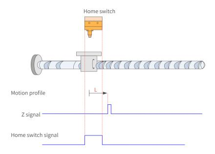
Figure 7-21 HW signal active at start
