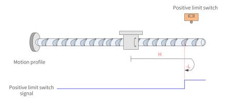
Figure 7-50 P-OT signal inactive at start
