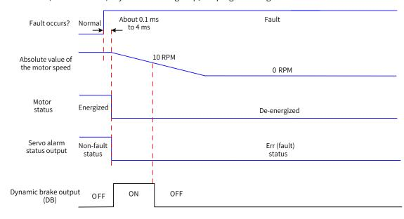
Figure 5-12 Timing diagram of "Dynamic braking stop, keeping de-energized status" at No. 1 fault (without brake)
