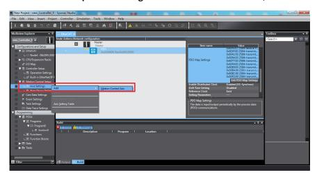
**MC\_Axis000** can be renamed through a simple click. For example, if it is named as Rewind axis, the axis variable Rewind axis used in the NX program represents control on this SV660N servo axis.
