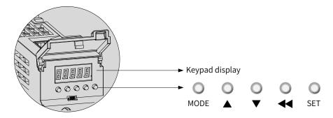
Figure 4-1 Appearance of the LED keypad
