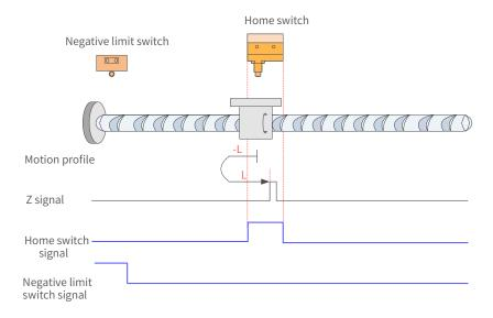
Figure 7-44 HW signal active at start
