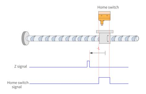
Figure 7-17 HW signal active at start
