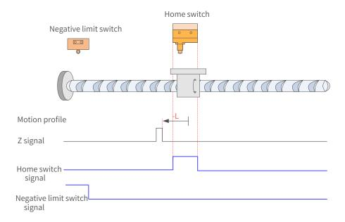
Figure 7-47 HW signal active at start
