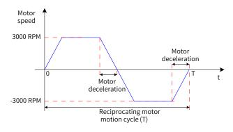
Figure 5-6 Motor speed curve without external load torque
