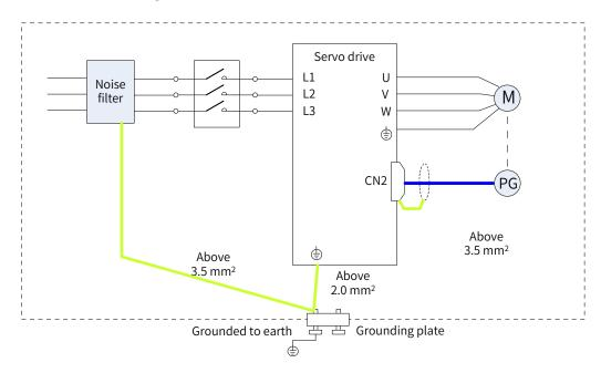
Figure 3-26 Anti-interference wiring example
