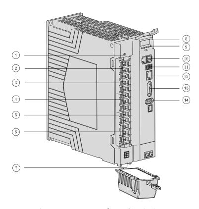
Figure 1-6 Components of servo drives in size E
