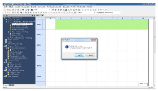
Click **Yes** and the coordinate transformation dialog box opens. Set mechanical parameters and the coordinate unit based on actual conditions and click **Execute calculation**. The software calculates the denominator and numerator for coordinate transformation automatically and writes parameters to **Axis control setting** automatically.
