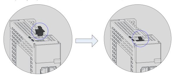
Figure 2-8 Mounting of the dust-proof cover
