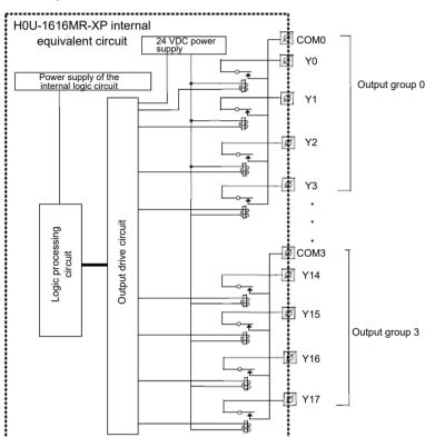
The following figure shows the internal equivalent circuit of mixed output of transistor and relay. Output terminals are divided into several groups, with each group electrically isolated. The output contacts of different groups are connected to different power circuits. Transistor output can be applied only to 24 VDC load circuit.
