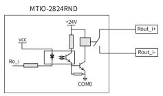
1) Electric shock protection when using inductive load
