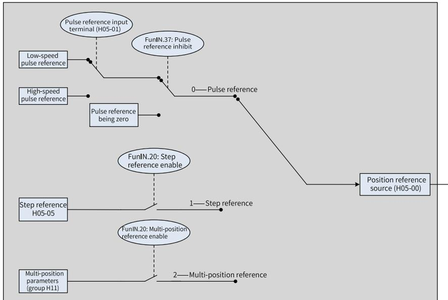
Figure 2-4 Setting the position reference source
