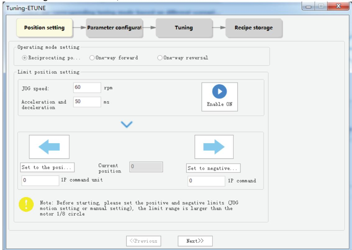
2. Select any of the following three operation modes based on the operating direction allowed by the machine.
