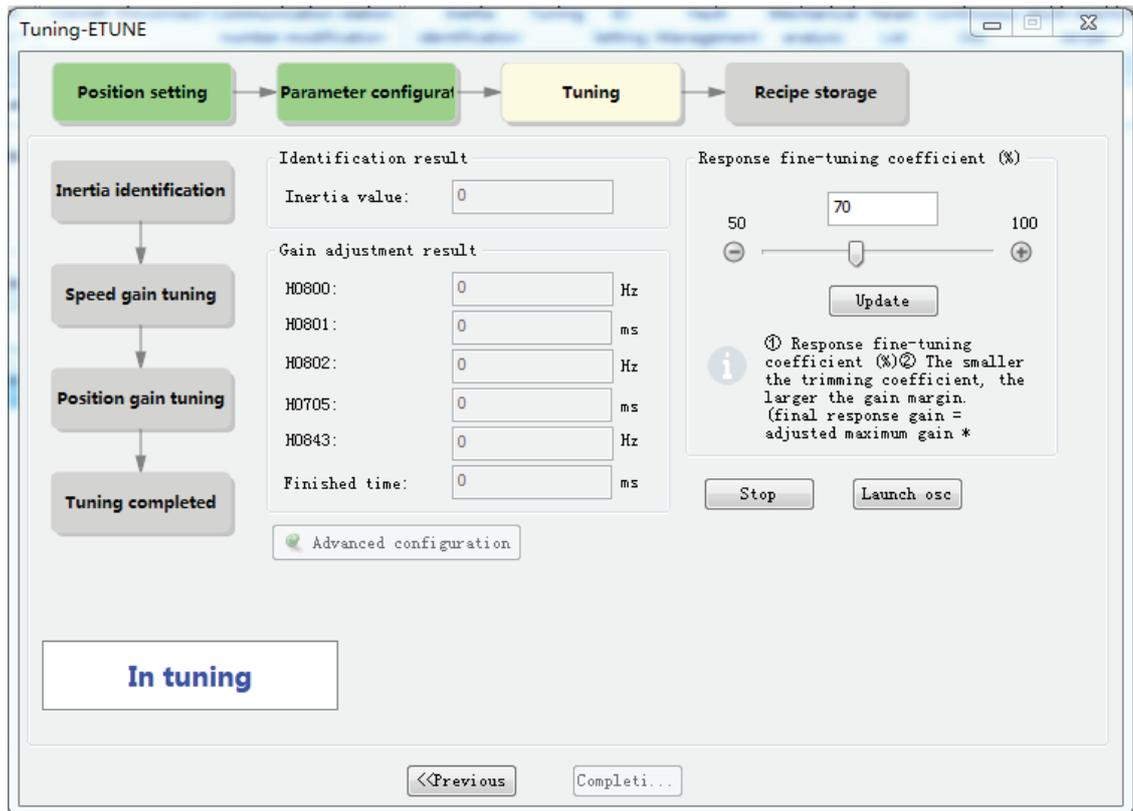
6. During gain tuning, if you modify the **Response fine-tuning coefficient** and click the **Update** button, gain tuning will be continued based on the fine-tuning coefficient required. After gain tuning is done, you can click the **DONE** button to save the parameters to EEPROM and export parameters as a recipe file.
