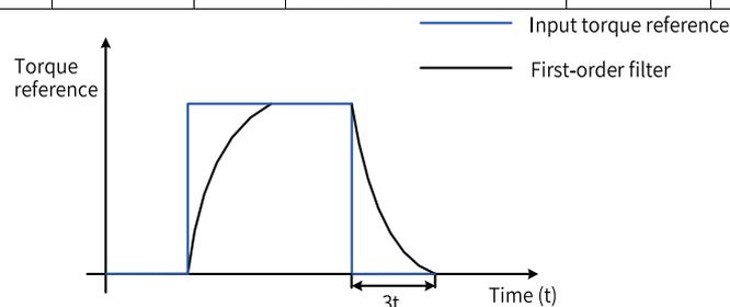
Figure 2-64 First-order filtering of rectangular torque references
