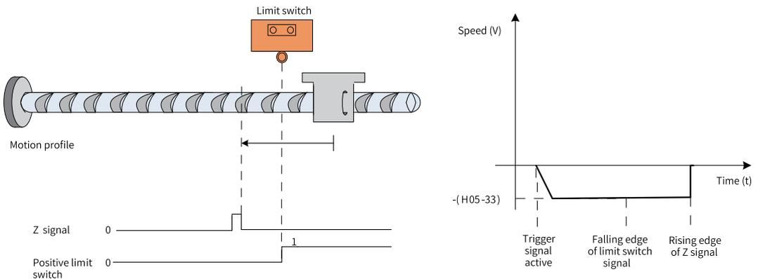
Figure 2-38 Motor operating curve and speeds in Mode 8
