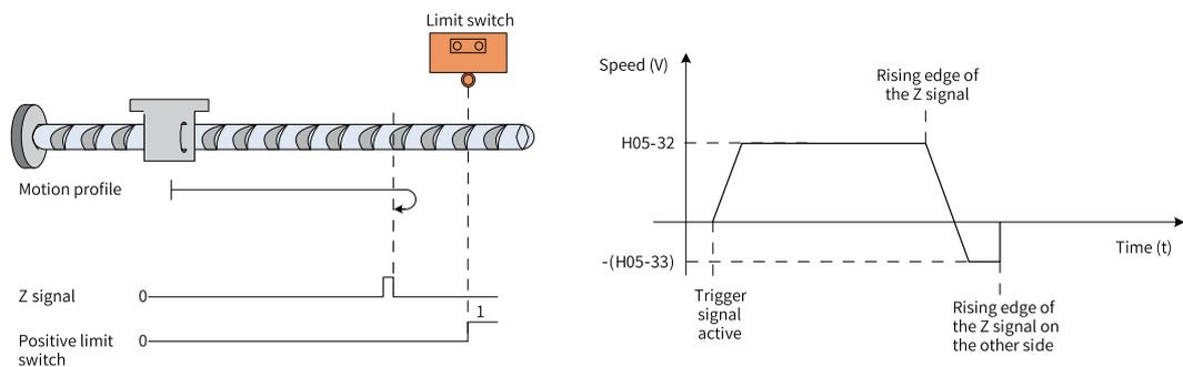
Figure 2-29 Motor operating curve and speeds in Mode 2
