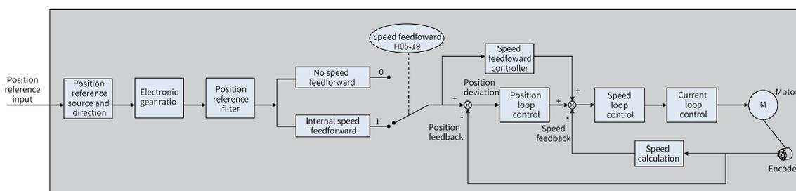
Figure 3-10 Operation diagram of speed feedforward control
