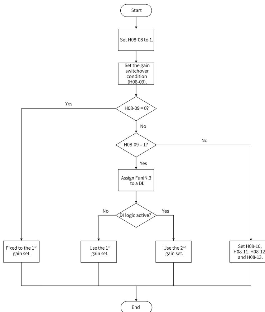
Figure 3-9 Gain switchover flowchart (H08-08 = 1)
