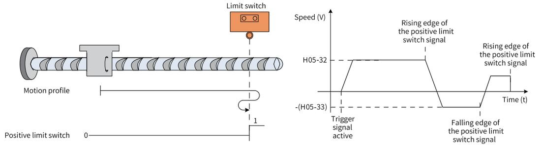
Figure 2-35 Motor operating curve and speeds in Mode 6
