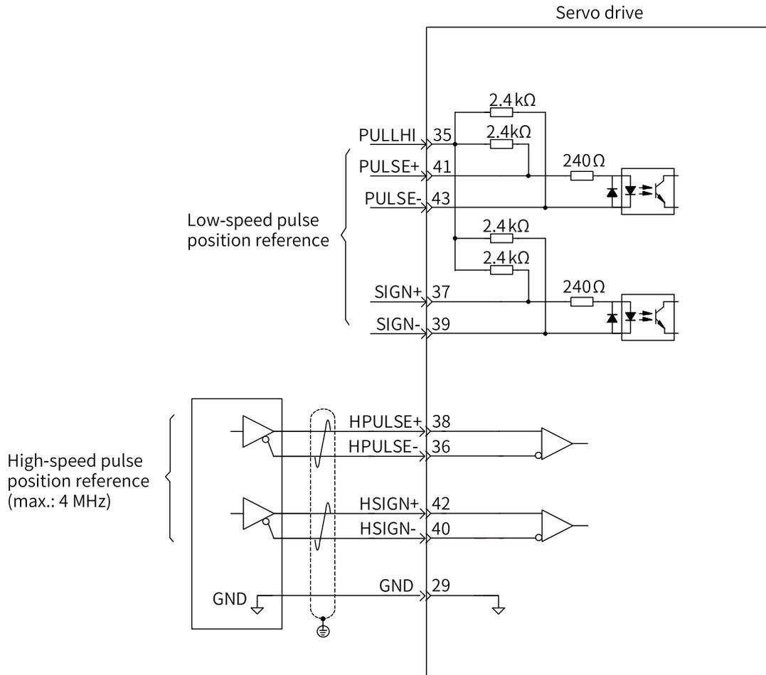
The low-speed pulse input terminals (PULSE+, PULSE-, SIGN+, SIGN-) receive differential input (maximum frequency up to 200 kpps) and open-collector input (maximum frequency up to 200 kpps).
