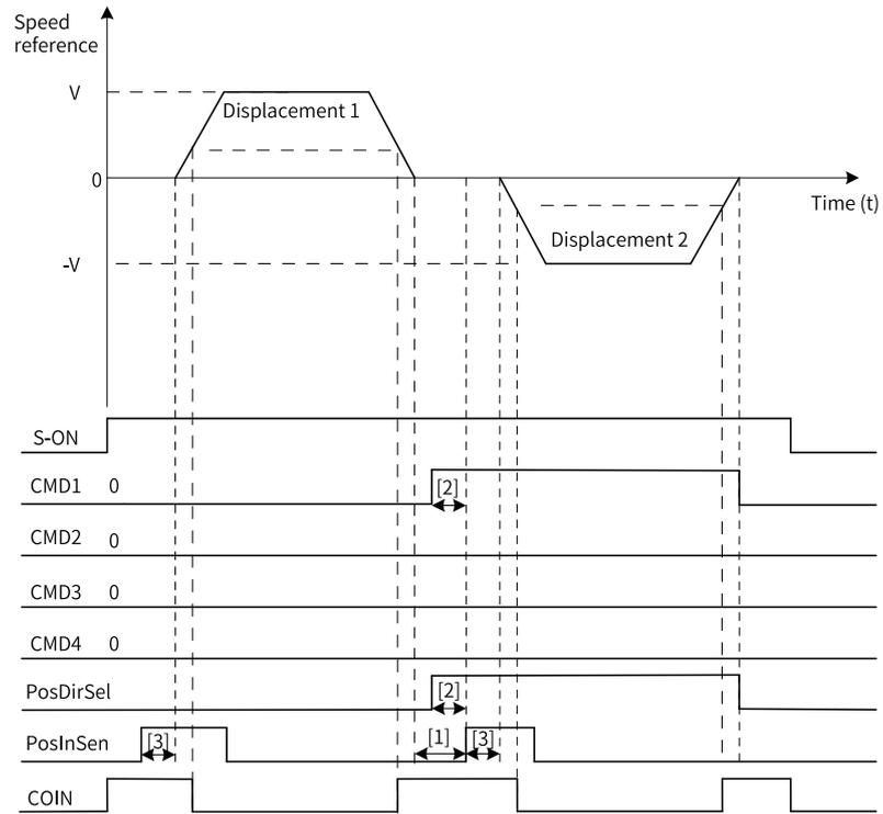
Figure 2-10 Multi-position sequence diagram
