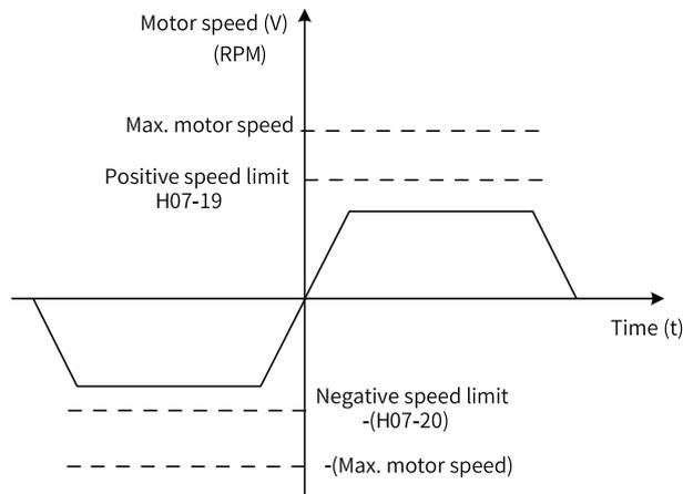
Figure 2-73 Speed limit curve (H07-17 = 0)
