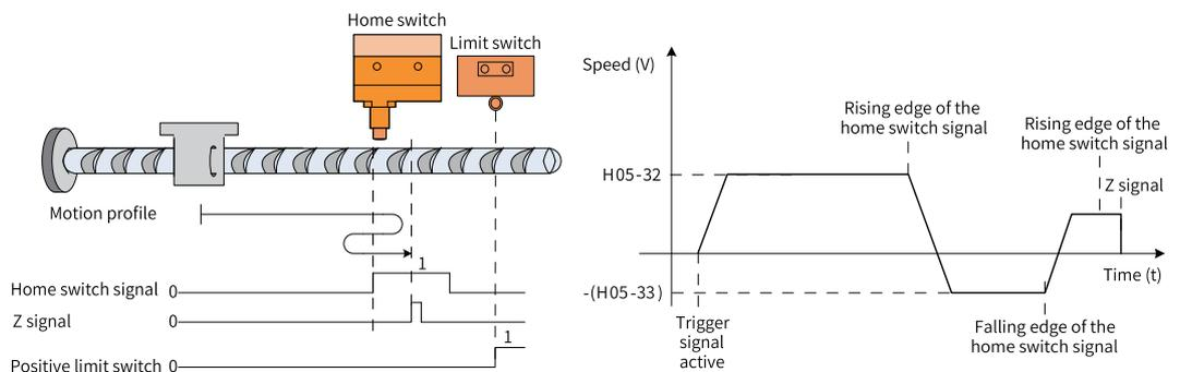
Figure 2-32 Motor operating curve and speeds in Mode 4
