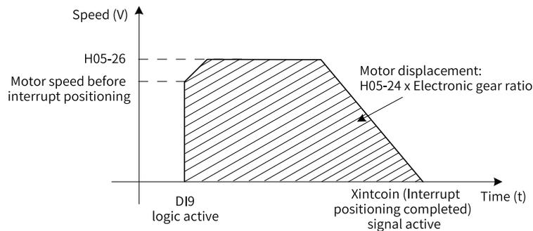
Figure 2-25 Motor operating curve during interrupt positioning
