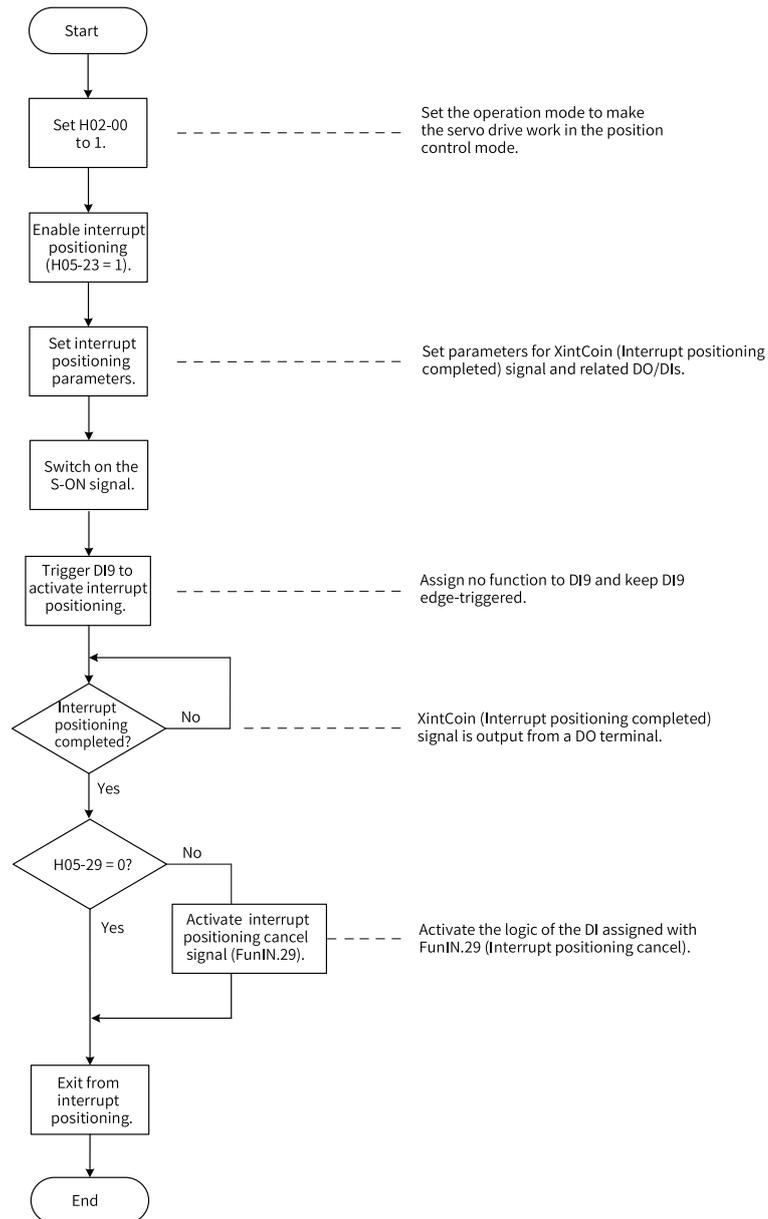
Figure 2-24 Flowchart of interrupt positioning signal
