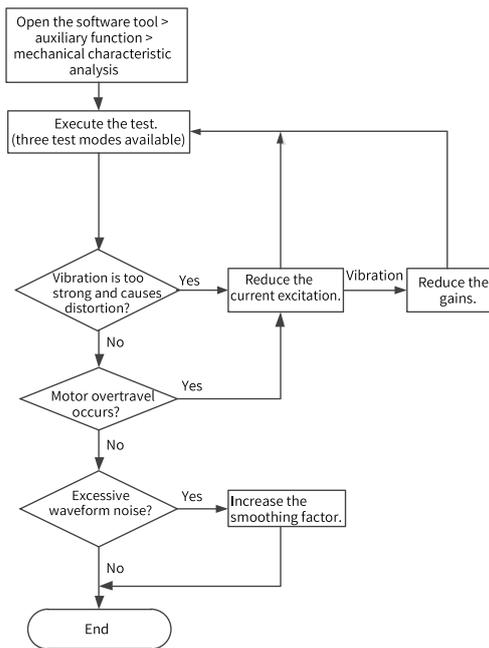
Figure 3-20 Operating procedure for mechanical characteristic analysis
