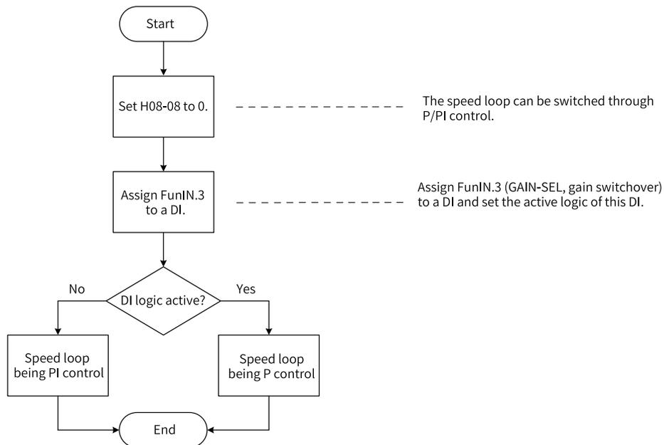
Figure 3-8 Gain switchover flowchart (H08-08 = 0)
