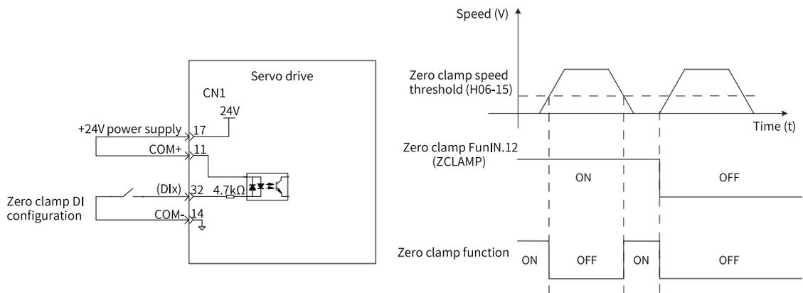
Figure 2-53 Wiring and waveform of zero clamp
