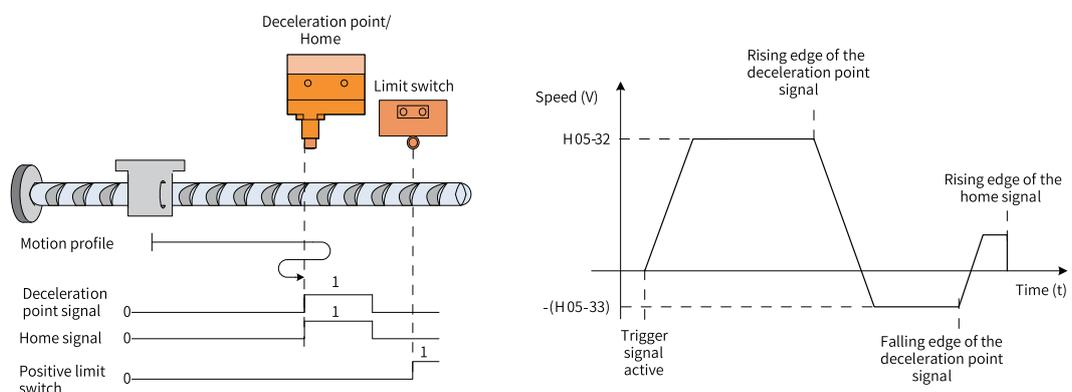
Figure 2-26 Motor operating curve and speeds in Mode 0
