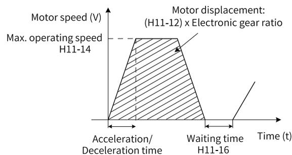
Figure 2-11 Motor operating curve in displacement 1
