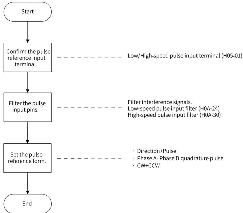
Figure 2-5 Flowchart for setting the pulse reference as the source
