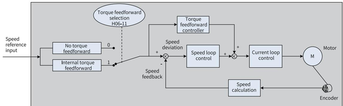
Figure 3-11 Operation diagram of torque feedforward control
