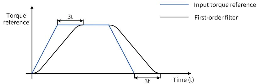
Figure 2-65 First-order filtering of trapezoid torque references
