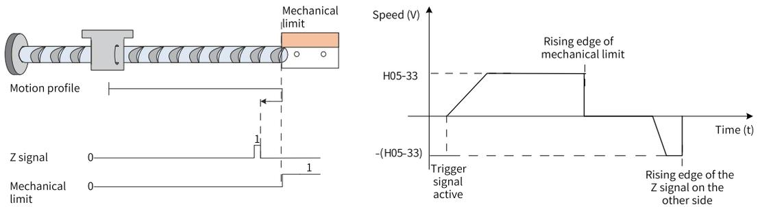
Figure 2-40 Motor running curve and speeds in Mode 12
