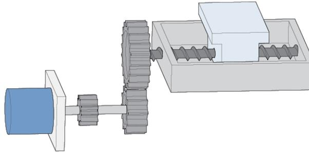
Figure 2-78 Ball screw transmission mechanism
