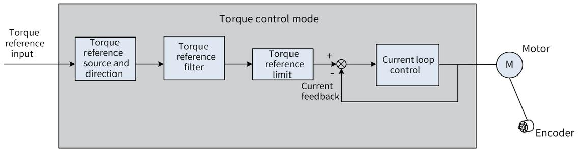
Figure 2-60 Block diagram of torque control mode
