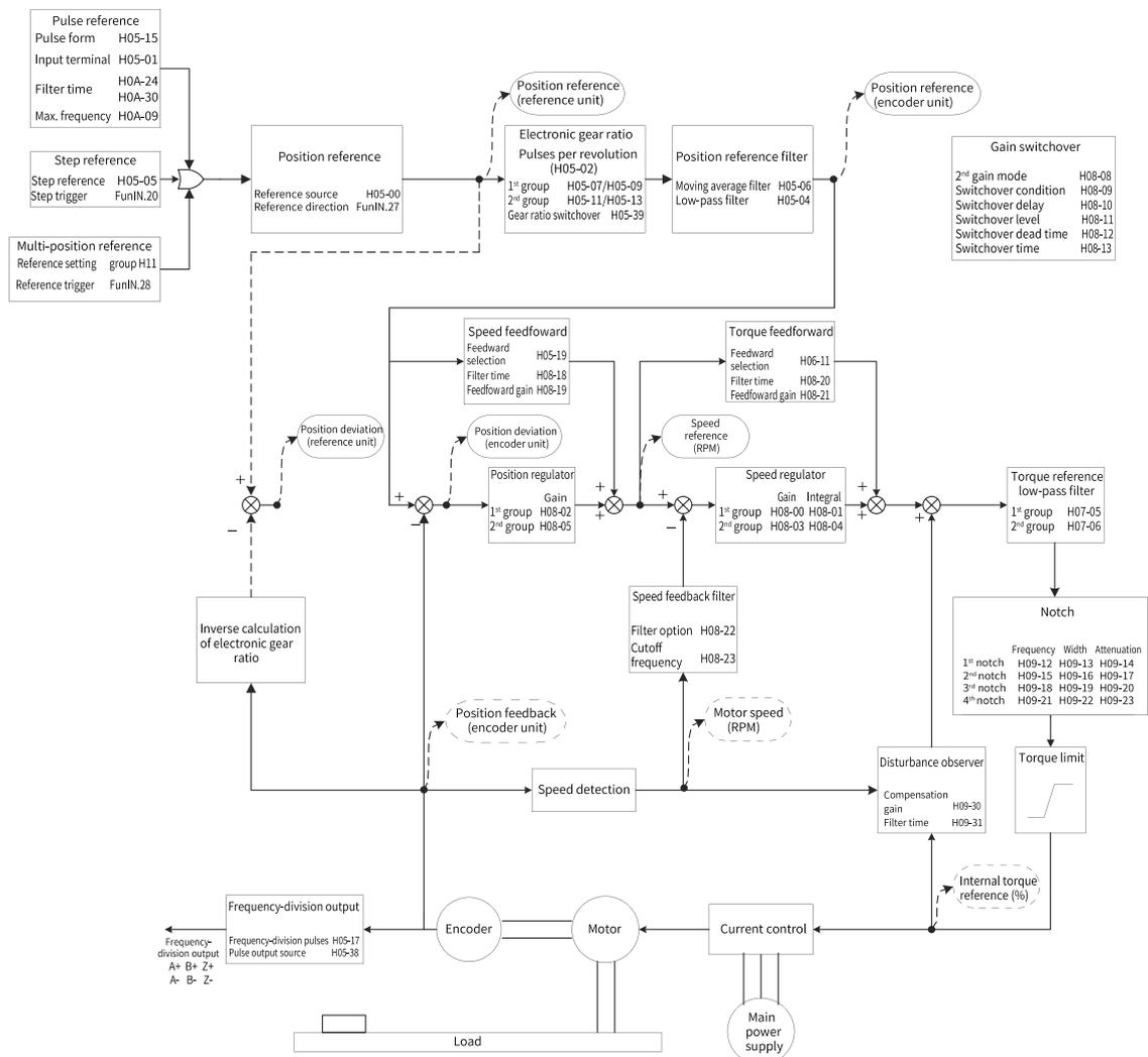
Figure 2-43 Block diagram of position control parameters
