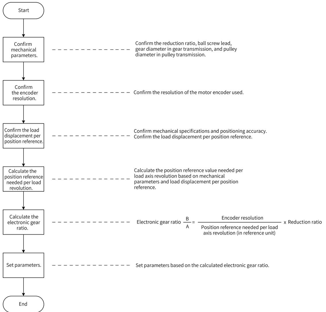
Figure 2-14 Procedure for setting the electronic gear ratio
