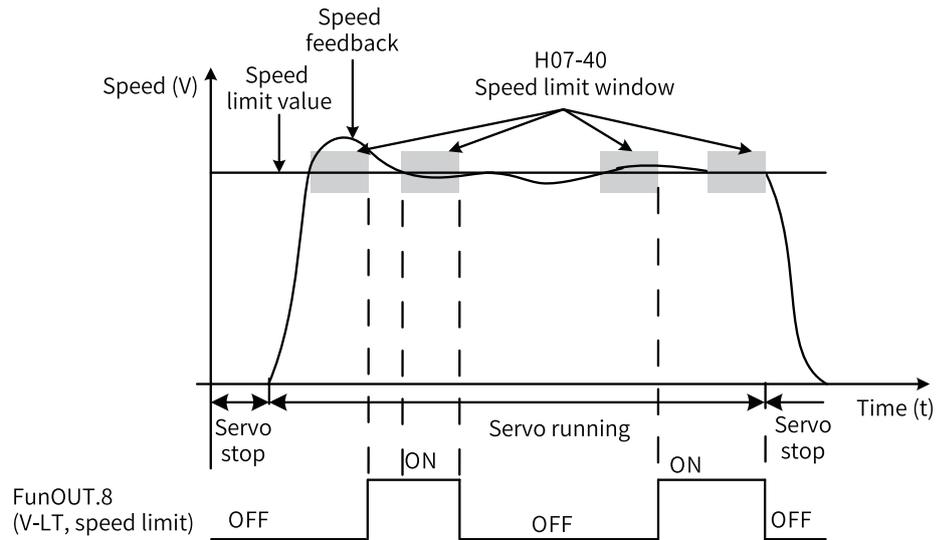
Figure 2-74 Example of speed limit DO waveform
