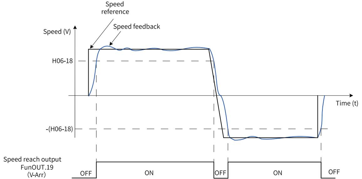
Figure 2-57 V-Arr signal waveform
