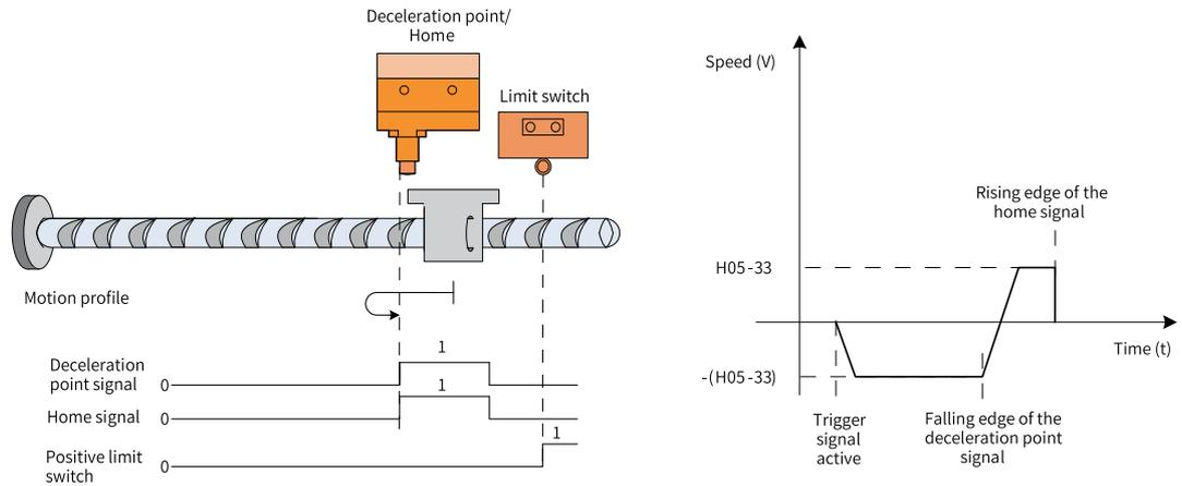
Figure 2-27 Motor operating curve and speeds in Mode 0
