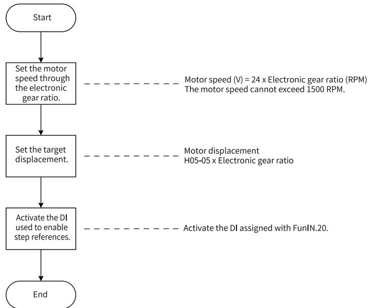
Figure 2-7 Flowchart for setting step reference
