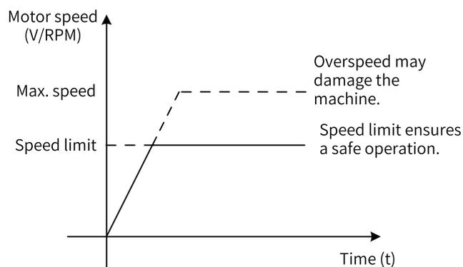
Figure 2-71 Speed limit in the torque control mode
