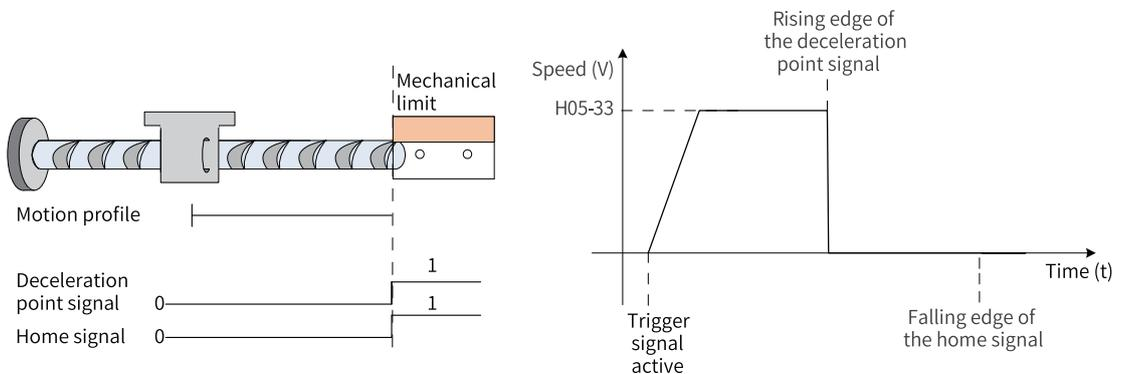
Figure 2-39 Motor operating curve and speeds in Mode 10
