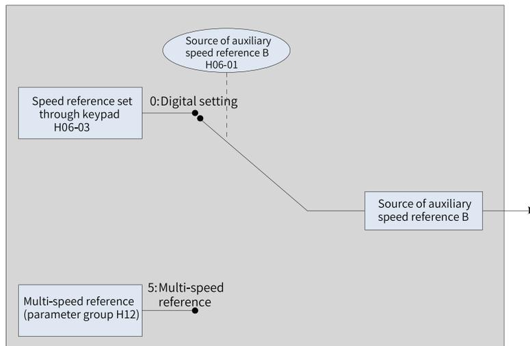
Figure 2-48 Source of auxiliary speed reference B
