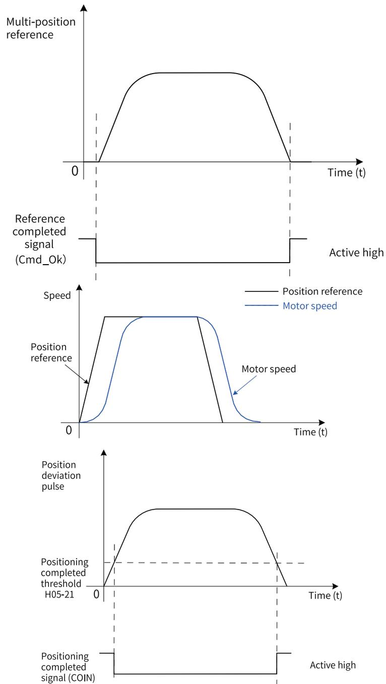
Figure 2-21 Description of positioning completed/proximity
