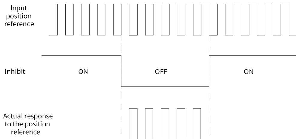
Figure 2-12 Example of position reference inhibition waveform
