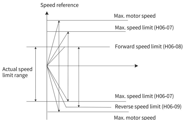
Figure 2-54 Example of speed reference limit
