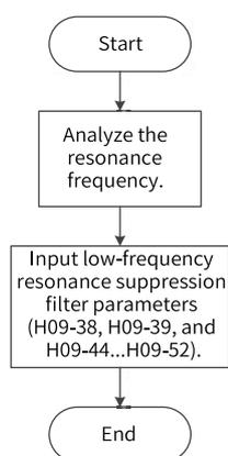
Figure 3-18 Procedure for setting low-frequency resonance suppression filter
