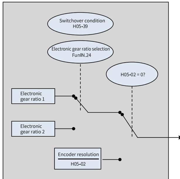
Figure 2-15 Procedure for setting the electronic gear ratio
