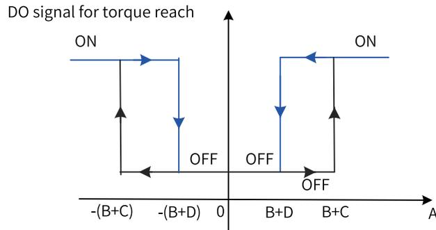
Figure 2-76 Active TorReach signal
