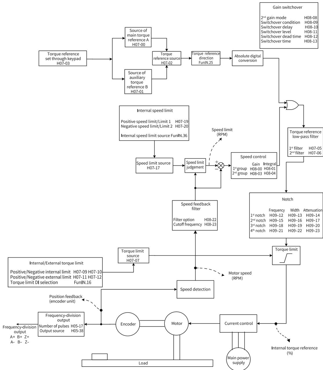
Figure 2-77 Block diagram of torque control parameters
