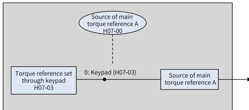
Figure 2-63 Source of main torque reference A
