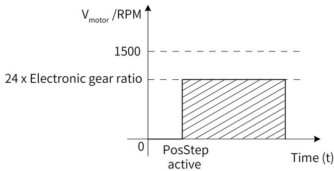
Figure 2-8 Motor operating curve (H05-00 = 1)
