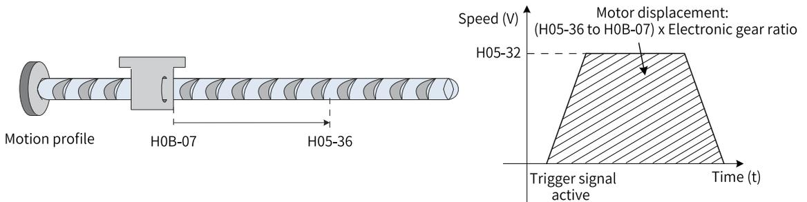
Figure 2-41 Motor operating curve and speeds in electrical homing
