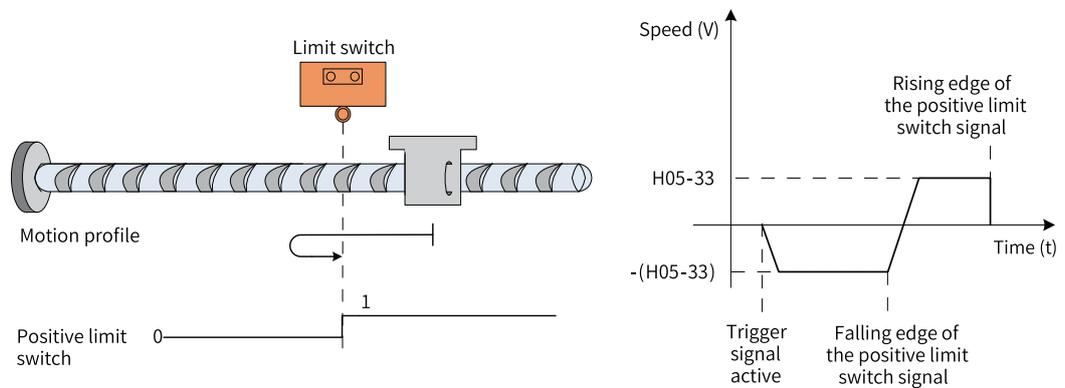
Figure 2-36 Motor operating curve and speeds in Mode 6
