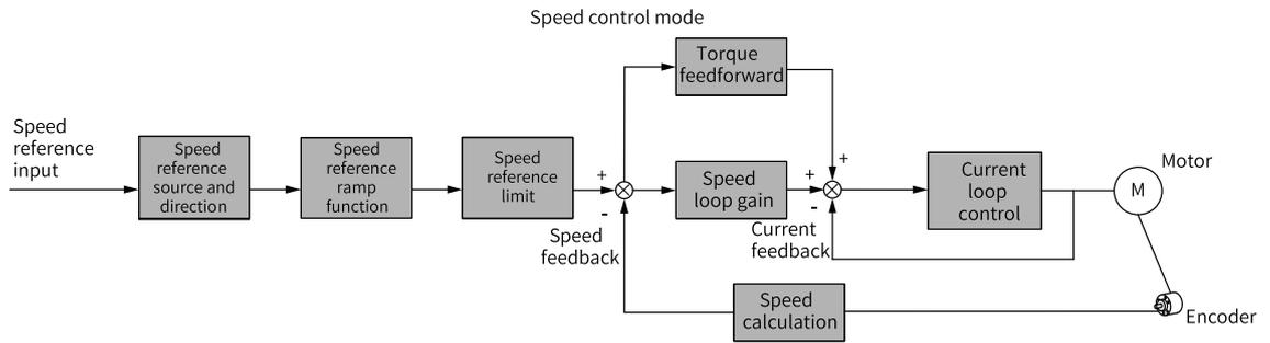
Figure 2-44 Speed control mode
