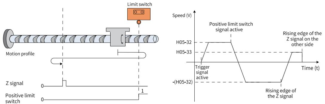
Figure 2-31 Motor operating curve and speeds in Mode 2
