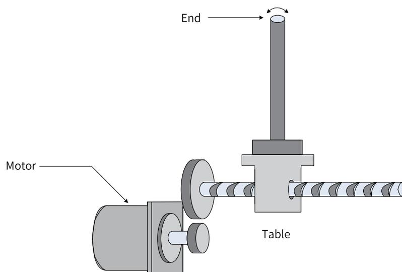
Figure 3-17 Low-frequency vibration at the mechanical load end
