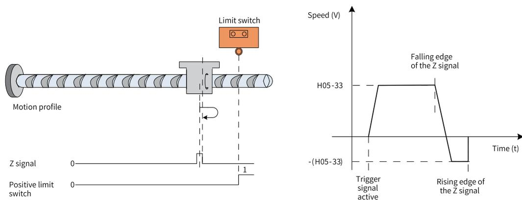
Figure 2-30 Motor operating curve and speeds in Mode 2
