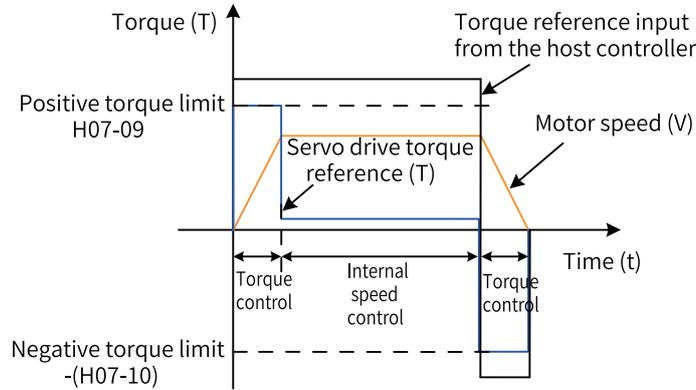
Figure 2-69 Torque limit curve (H07-07 = 0)
