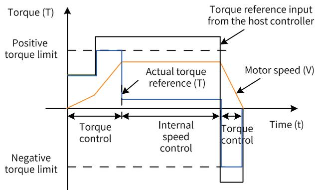
Figure 2-66 Torque reference and torque limit
