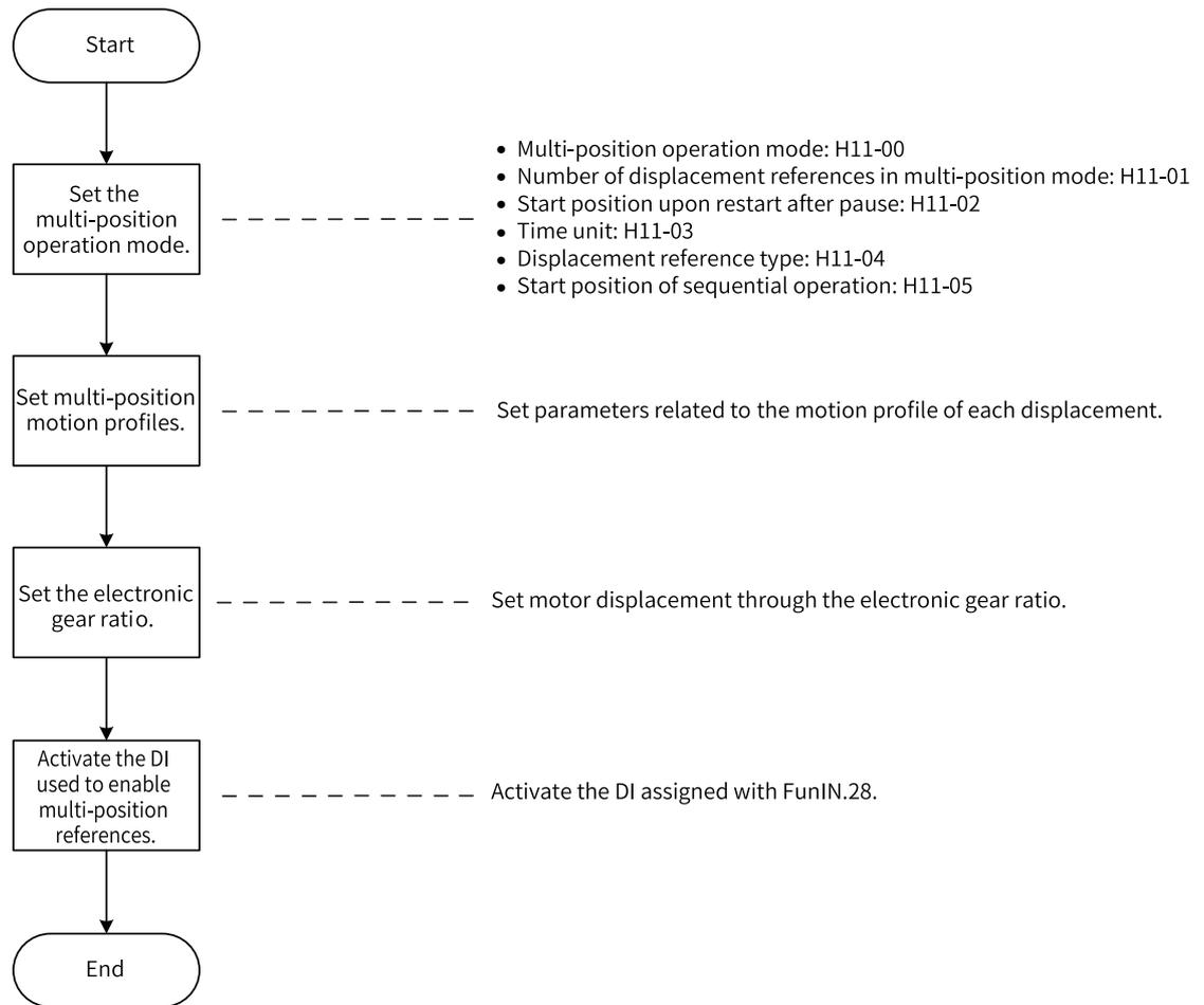
Figure 2-9 Flowchart for setting multi-position reference as the source
