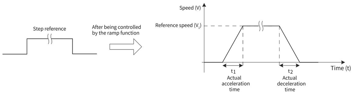
Figure 2-52 Definition of the ramp function
