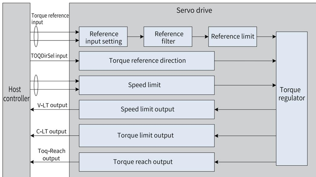
Figure 2-61 Signal exchange between the servo drive and the host controller
