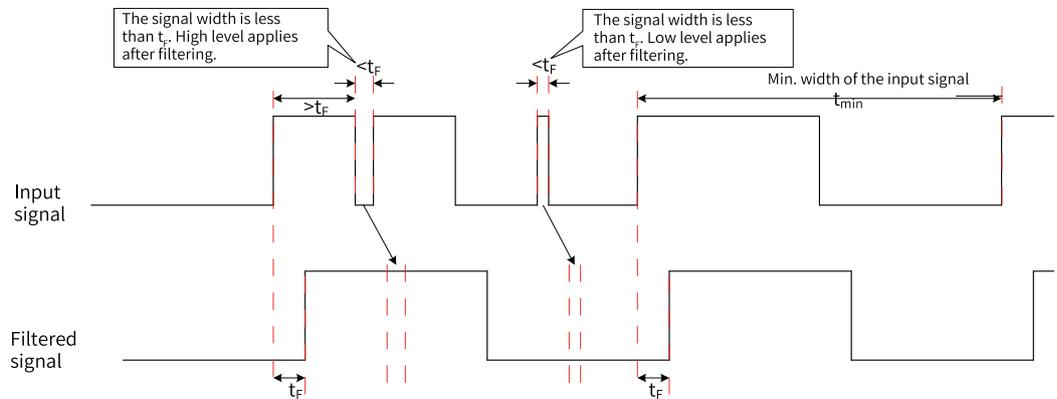
Figure 2-6 Example of filtered signal waveform
