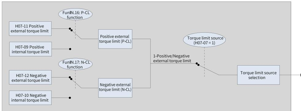
Figure 2-70 Torque limit source (H07-07 = 1)
