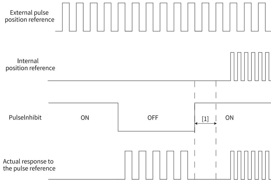
Figure 2-13 Waveform example for pulse reference inhibit
