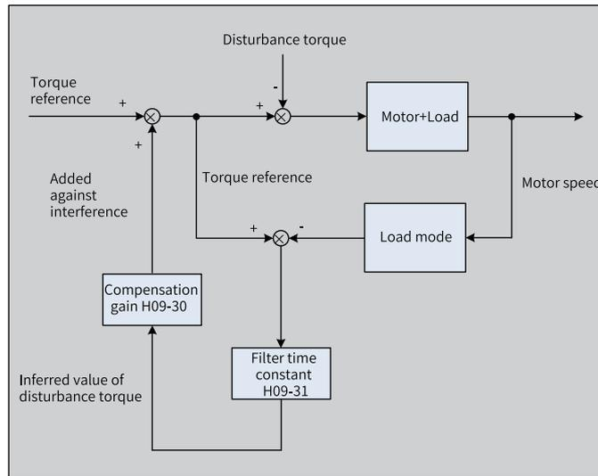
Figure 3-13 Block diagram for disturbance observer 2
