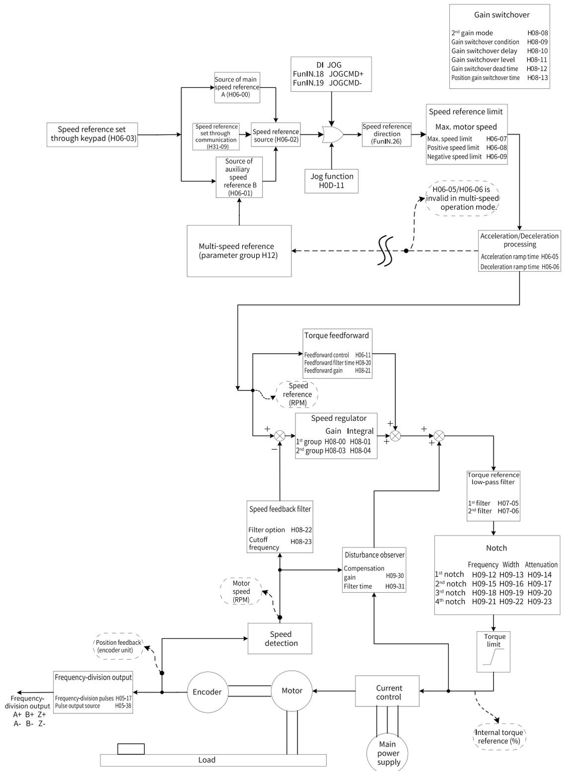
Figure 2-59 Block diagram of speed control parameters
