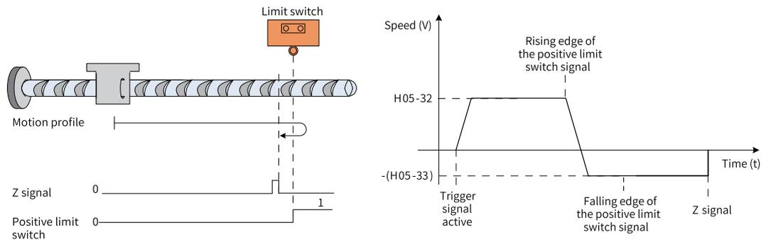
Figure 2-37 Motor operating curve and speeds in Mode 8
