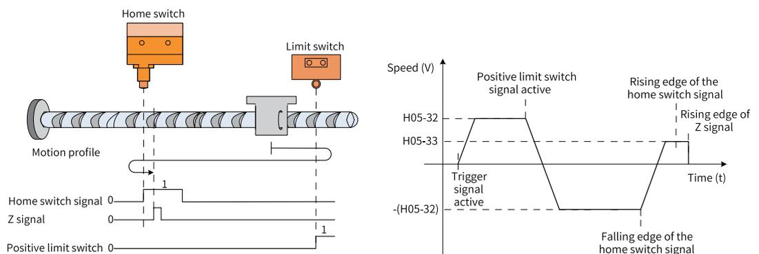
Figure 2-34 Motor operating curve and speeds in Mode 4
