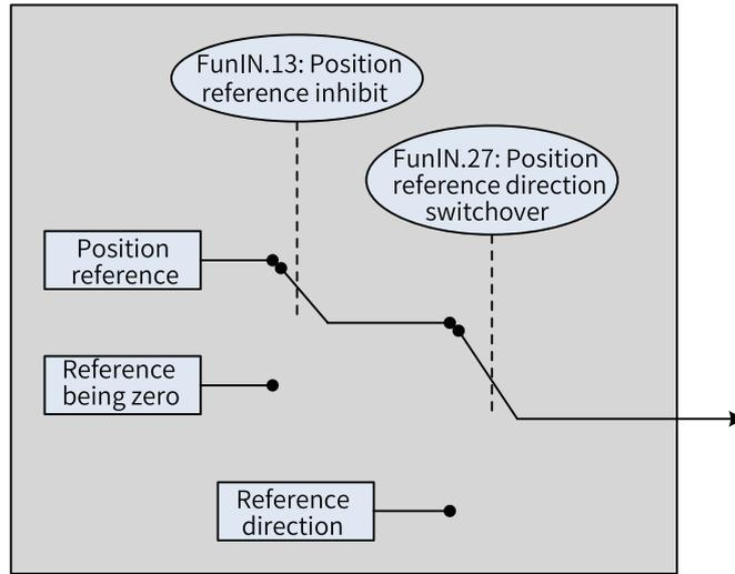
Figure 2-3 Position reference input setting
