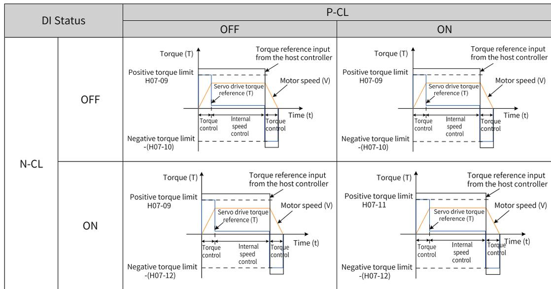
Assign FunIN.16 (P-CL: Positive external torque limit) and FunIN.17 (N-CL: Negative external torque limit) to two DIs and set the active logic of these two DIs.
