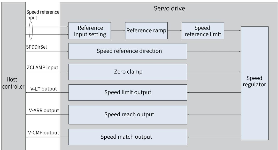
Figure 2-45 Signal exchange between the servo drive and host controller
