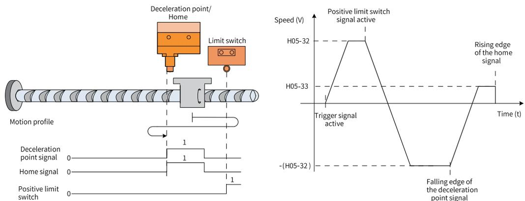
Figure 2-28 Motor operating curve and speeds in Mode 0
