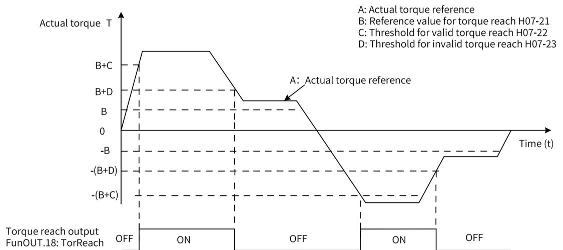
Figure 2-75 Example of torque reach output waveform
