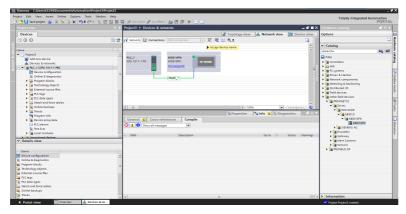
5) Connect the device correctly, allocate a device interface, and click Update list.
