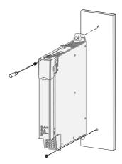
Figure 2-10 Backplate mounting of 22 kW power supply unit (50 mm wide)
