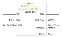
REQ: Command enabled. Diagnosis information reading is enabled when it is set to ON.
