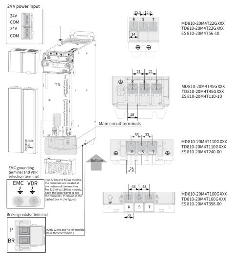
Figure 3-1 Assignment and dimensions of terminals in power supply unit (booksize, unit: mm)
