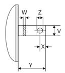
Figure 9-23 Dimensions of the copper bar(unit: mm)
