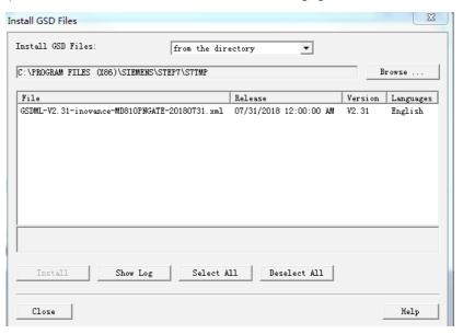
If the import is successful, the device is displayed, as shown in the following figure.
