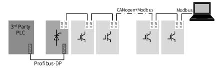
Figure 6-12 Communication networking of switching the PROFIBUS-DP to the CANopen network bridge
