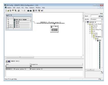
Step 4: Configure PROFIBUS-DP slave parameters. Double-click the MD810 slave, as shown in the following figure:
