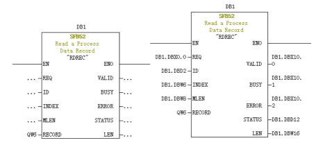
In the preceding figure, default parameters are used on the left, that is, parameters are set according to the information shown on the right. You can customize parameters or use default parameters for corresponding blocks as required. However, if multiple invocations are involved, you need to customize parameters to avoid invocation errors caused by default parameters (note: RECORD must be customized).
