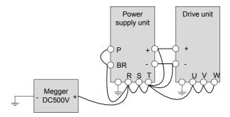
Figure 8-1 Test insulation on the main circuit
