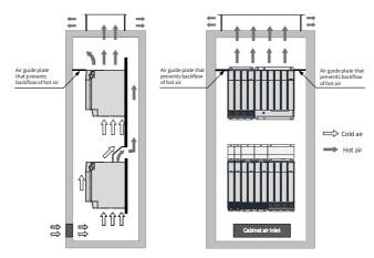
Figure 2-7 Backflow of hot air in the passive air discharge cabinet (with an isolating device)
