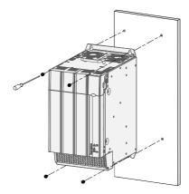
Figure 2-12 Backplate mounting of 110kW power supply unit (200mm wide)
