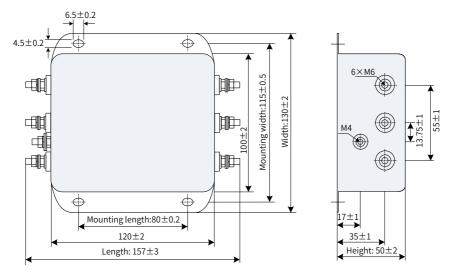
Figure 9-27 Mounting dimensions of the simple EMC filter (unit: mm)
