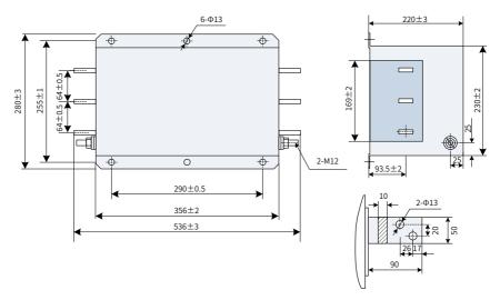
Figure 9-26 Dimensions of Jianli series filter of 1000 A (unit: mm)
