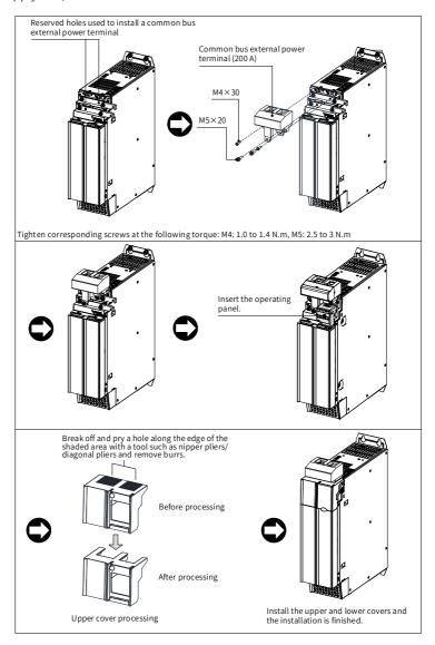
■ Installation example of 200 A common bus external power terminal (110 kW and 160 kW power supply units)
