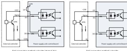
Sink connection method using the internal 24 V power supply of the power supply unit
