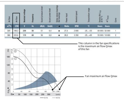
Figure 2-8  $\,Q_{max}$  of a system fan
