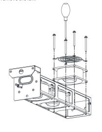
■ Installing the fan of a vertical tower unit
