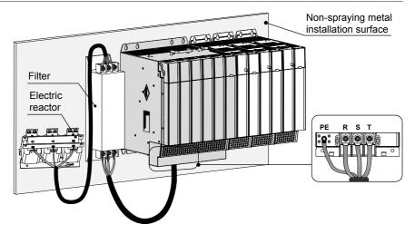
Figure 3-3 Protective grounding connection of main circuit terminals
