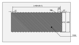
Figure 9-3 Physical appearance of the embedded mounting bracket and backplate tapping dimensions (unit: mm)
