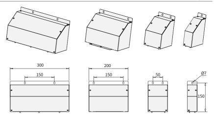
Figure 9-4 Overall dimensions of the heat insulation baffle (unit: mm)
