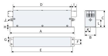
Figure 9-21 Dimensions of Schaffner FN 3258 series filter of 50 to 180 A (unit: mm)
