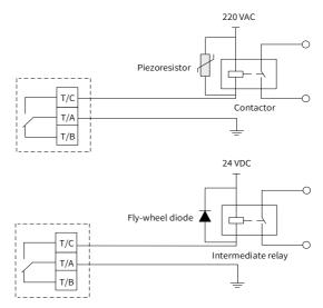
Figure 3-13 Anti-interference processing of relay output terminals
