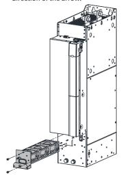
4) Loosen four screws from each fan cover and remove the fan.
