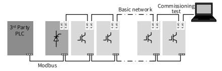
Figure 6-1 Modbus communication networking
