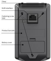
Figure 4-5 Appearance of external LCD operating panel
