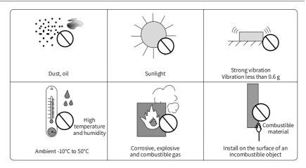
Figure 2-1 Installation environment
