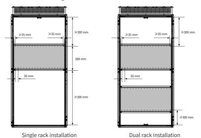
■ Dimensions of mounting holes of vertical tower unit (355 kW power supply unit)
