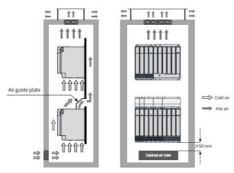
Figure 2-5 Position of the cabinet air inlet
