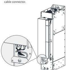
Remove two screws from the fan box and draw the fan box out in the direction of the arrow.
