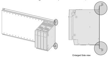
■ Scheme 2: A lateral reinforced beam is welded on the back of the backplate.
