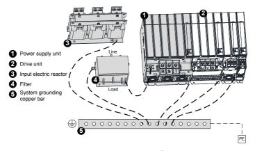
Figure 3-7 System protective grounding connection
