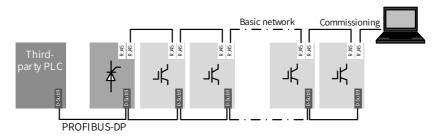
Figure 6-9 PROFIBUS-DP communication networking
