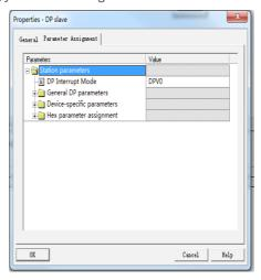
Parameters PZD1 to PZD12 are for customized periodic data exchange. They can be configured in hardware configuration. Double-click the MD810DP sign in HW Config, click "Device-specific parameters", and configure corresponding parameter addresses as required.
