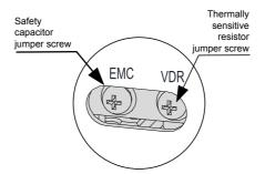
Figure 8-2 Positions of ground jumpers of the VDR screw and EMC screw For details, see "Figure 3-1 Assignment and dimensions of terminals in power supply unit (booksize, unit: mm)" and "Figure 3-2 Assignment and dimensions of terminals in power supply unit (vertical tower, unit: mm)".
