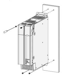
Figure 2-11 Backplate mounting of 45 kW power supply unit (100 mm wide)
