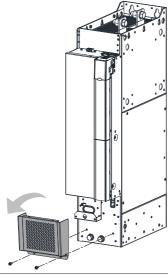
2) Disconnect the fan power cable connector from the power supply unit. Each fan has a power
