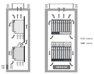
Figure 2-6 Backflow of hot air in the passive air discharge cabinet (without any isolating device)
