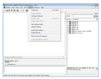
Click Install. After the installation is finished, the MD810-gateway module will emerge under Gateway, as shown in the following figure:
