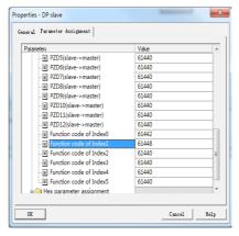
After all the preceding operations are complete, the PROFIBUS slave station is configured. Now, you can compile programs in S7-300 to control the drive.
