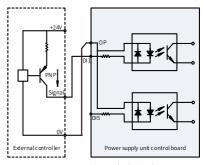
Source connection method using the external 24 V power supply
