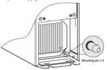
2) Insert the two guide pins into the square holes and then press in the hook.
