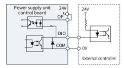
Figure 3-14 DO terminal wiring
