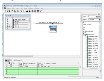
Step 5: Configure INPUT and OUTPUT data length.
