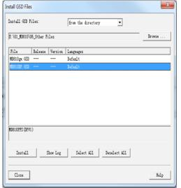
Click Install. After installation is complete, the PROFIBUS-DP module of MD810DP is displayed, as shown in the following figure.
