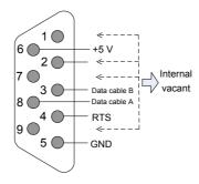
Figure 6-10 DB9 interface pins
