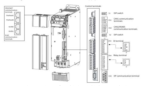
Figure 3-8 Assignment of control circuit terminals in the power supply unit
