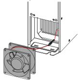
• Install the fan into the power supply unit and ensure that the mounting pins are aligned.
