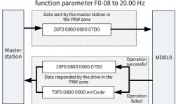
Master station changing the value of drive function parameter F0-08 to 20.00 Hz
