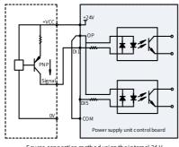
Source connection method using the internal 24 V power supply of the power supply unit
