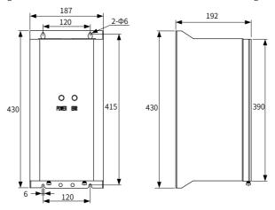
Figure 9-9 Overall dimensions of the MDBU series braking unit (unit: mm)
