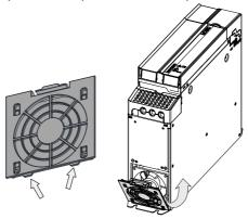
3) After the replacement is complete, check that the air flow direction is upright.
