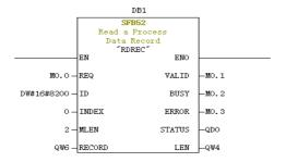
After M0.0 is set, the function block reads F0-02 (Index 0 has been set to F0-02 before) of the drive No. 3 and saves it in QW6. Field definitions are as follows:
