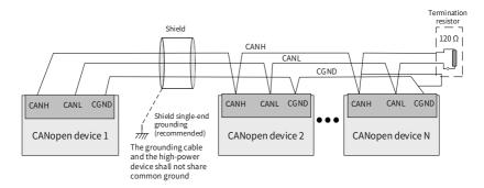
Figure 6-5 CAN bus connection topology
