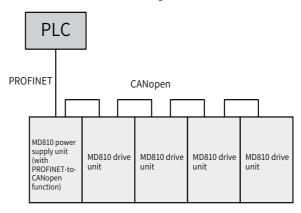
The network bridge function implements data exchange for a total of 30 nodes (including the power supply unit). Detailed data is as follows.
