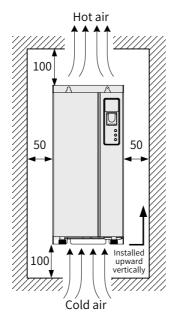
Figure 9-8 Installation dimensions of the MDBUN series braking unit
