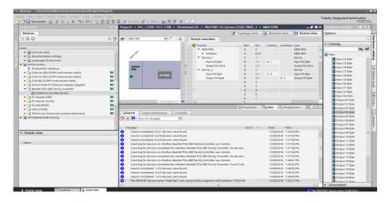
3) Download the configuration to the PLC. After the hardware configuration in step 2 is modified, download the configuration to the PLC again. If only the hardware configuration is modified, you can download only the hardware configuration.
