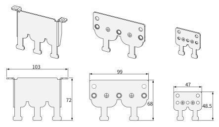
Figure 9-5 Overall dimensions of the shielded bracket (unit: mm)
