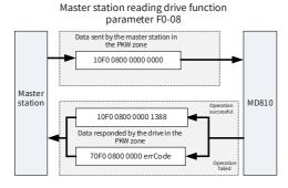
1) Example PKW data sent by the master station when reading a drive parameter
