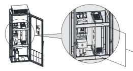
Upper and lower cross beams (selfmade according to an actual cabinet), fixed with six M6 screws for auxiliary fixing during cabinet transportation. They can be removed for recycling after arrival at the terminal site.
