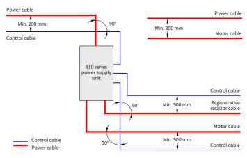
Figure 3-10 Cabling diagram
