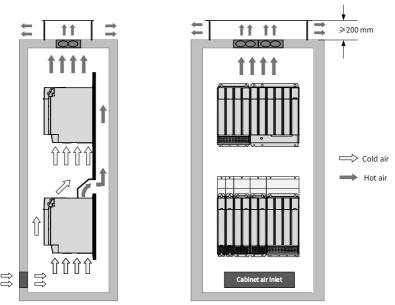
Figure 2-9 Cabinet exhaust air system of the power supply unit
