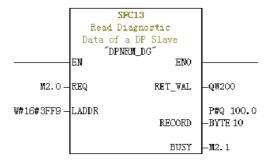
REQ: Command enablement. When this field is set to ON, diagnosis information reading is initiated.
