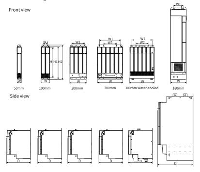
Figure 9-1 Overall dimensions of the power supply unit
