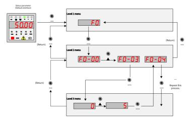
Figure 4-2 Operation flowchart for the 3-level menu structure
