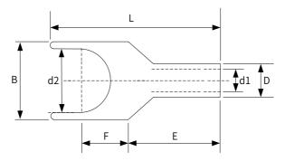
Figure 9-15 Dimensions of TNS series lug
