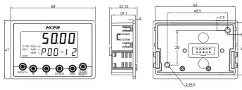
Figure 2-6 External dimension for LCD panel
