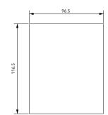
Figure 2-7 Cutout dimension for external keyboard and tray
