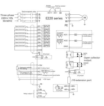
Figure 3-1 Typical wiring for inverter of three-phase 15kw or less
