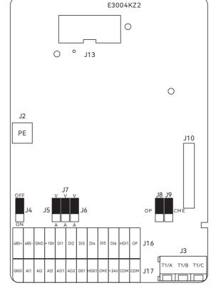
Figure 3-2 Terminal arrangement of control circuit
