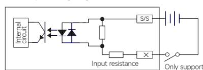
Figure 9 Local IO input wiring for HCO0-1200-D/1100-D
