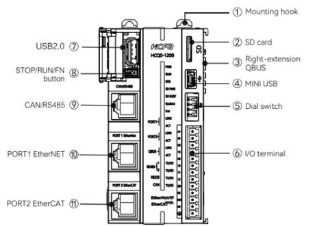
Figure 2 HCQ0-1200-D/1100-D CPU unit viewed from the front side
