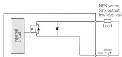
Figure 10 Local IO input wiring for HCO0-1200-D/1100-D
