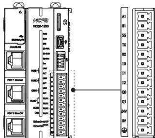
Figure 3 Terminal description for HCQ0-1200-D/1100-D
