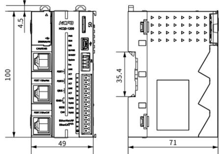
Figure 8 HCO0-1200-D/1100-D CPU installation dimension (unit: mm)
