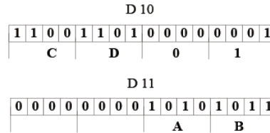
Bit composition when M8161 is OFF and n is 6 Conversion by using D100 to D102 (high- and low-order bytes)
