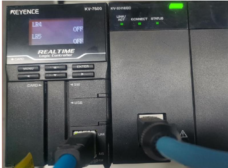
In the monitor state, click the item column [KV-XH16EC], open the unit monitor to view the Y7 servo, click [Test Run], and test run the servo shaft in different modes.
