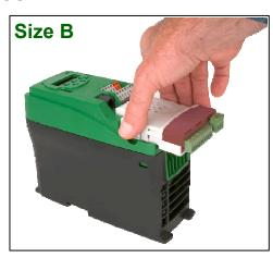
This "Encoder Speed Reference" input is not a true quadrature counter - therefore applications which require accuracy when operating close to zero speed will not be possible. Therefore, generally this option <u>cannot</u> be used for position applications but is more suited to applications that require accurate speed holding and speed following.
