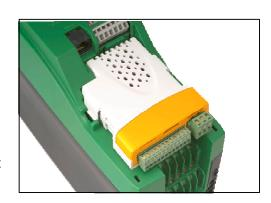
This "Encoder Speed Reference" input is not a true quadrature counter - therefore applications which require accuracy when operating close to zero speed will not be possible. Therefore, generally this option cannot be used for position applications but is more suited to applications that require accurate speed holding and speed following.
