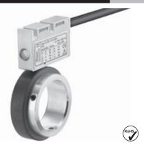
Thanks to its installation depth of only 16 mm, the bearingless magnetic rotary encoder RI20 / LI20, comprising a magnetic ring and sensor head, is ideally suited for plants and machinery where space is very tight. The non-contact measuring principle allows for error-free use even under harsh environmental conditions, as well as ensuring a long service life.
