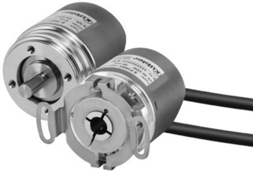
The Sendix F36 multiturn with the patented Intelligent Scan Technology™ is an optical multiturn encoder in miniature format, without gears and with 100% insensitivity to magnetic fields. With a size of just 36 x 42 mm it offers a shaft or a blind hollow shaft of up to 10 mm.
