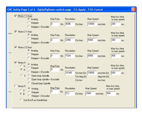
The ADV400 is capable of doing up to five axis.
