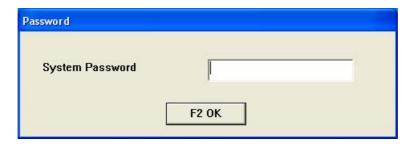
With no password (pressing F2), the system will be at machine User level. The User level permits to home the axis, to move manually the axis and to run the present part program.
