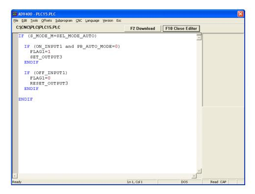
**Download** (or F2 on the keyboard) is sending the PLC to the controller and automatically uses it (like the Load button on the Managing PLC page)
