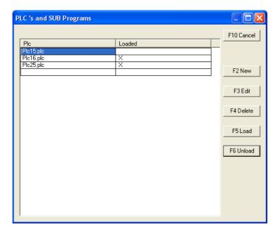
**New** (or F2 on the keyboard) permits to create a new custom PLC (opening text editor with blank page).
