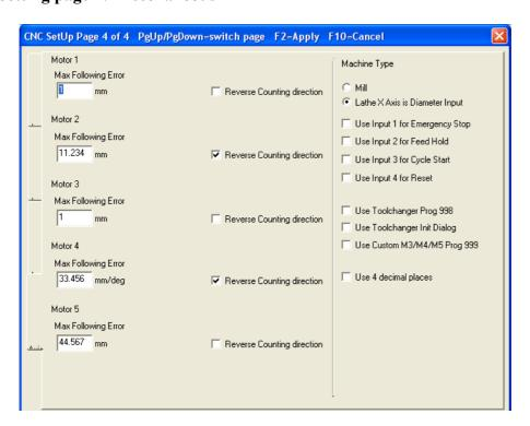
This page permits to indicate the **Maximum Following Error** allowed for an axis, in millimeters.
