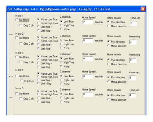
If an axis is used (check box activated in Setting page 1), the informations on this page must be entered.
