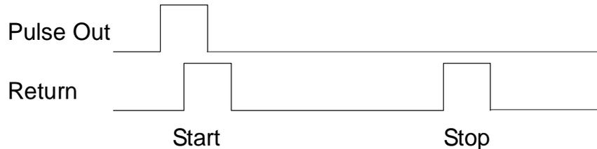
**Figure 14 RPM Signal Format**
