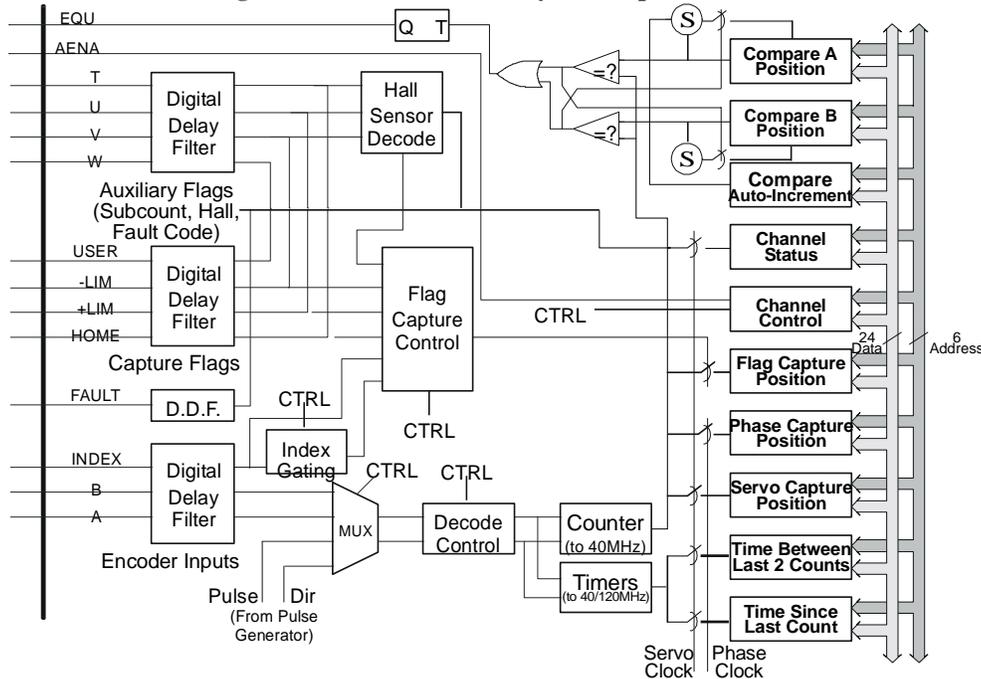
Figure 5 PMAC2 Gate Array IC Encoder/Flag Channel
