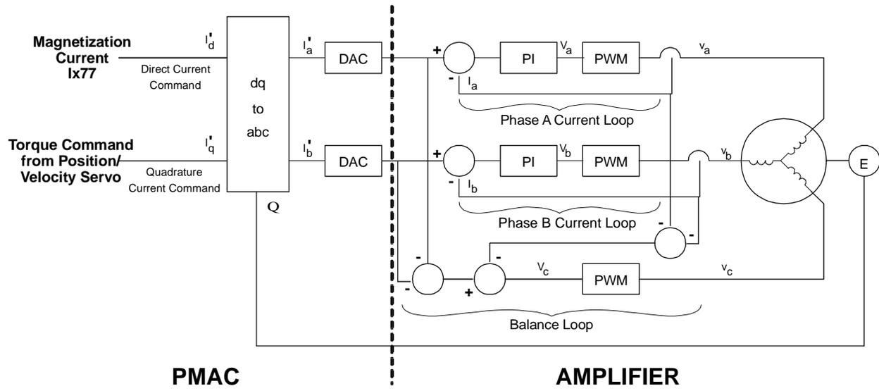
Figure 8 PMAC/PMAC2 Commutation with Analog Current Loop
