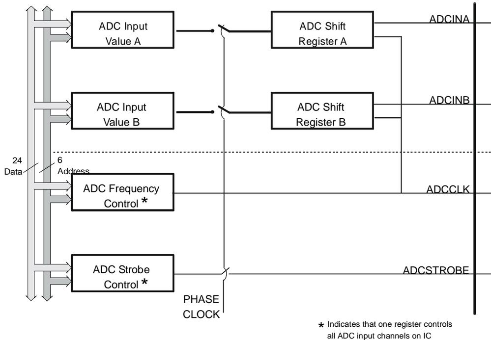
**Figure 6 PMAC2 Gate Array IC Input Channel**
