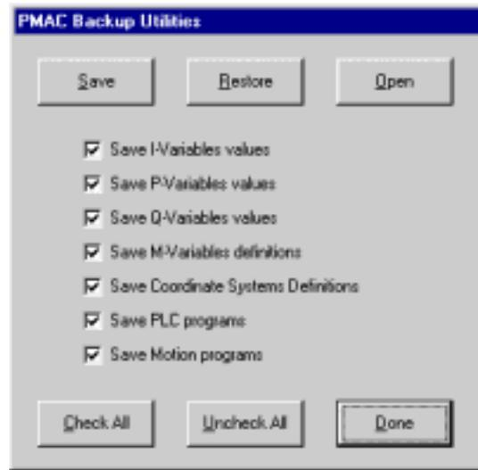
Once PMAC is properly configured, save the software parameters in a backup file. On this page, select the parameters to save and the name of the file.
