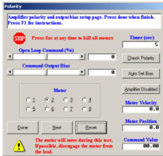
On this page, the motor polarity is checked. Correct polarity will show increasing encoder counts when PMAC outputs a positive command signal. This procedure requires the amplifier and motor being powered so, if possible, mechanically disengage the motor from the load.
