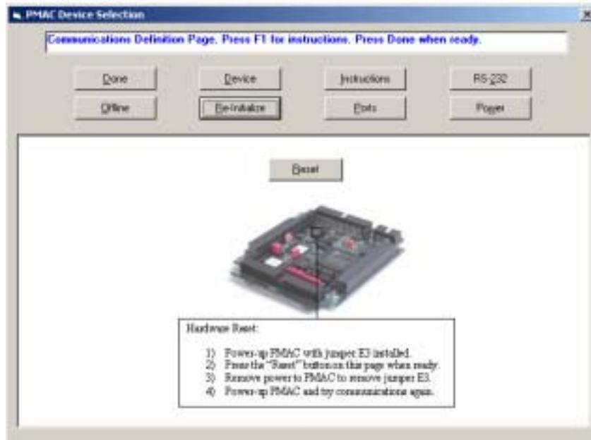
1. Press the **Re-Initialize** button on the Communications Setup screen.
